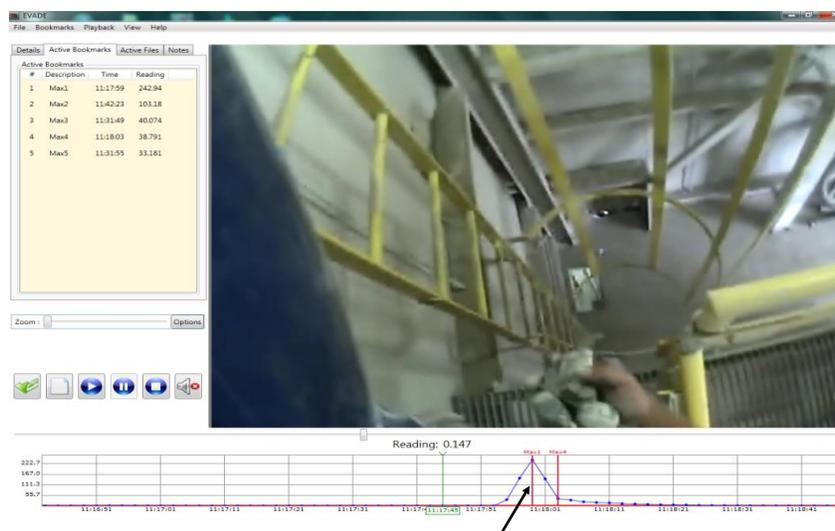
**Figure 9.8. EVADE screenshot with labels added to indicate respirable dust exposure to a worker from climbing down a ladder and exposure from dust released from ladder rungs.**
