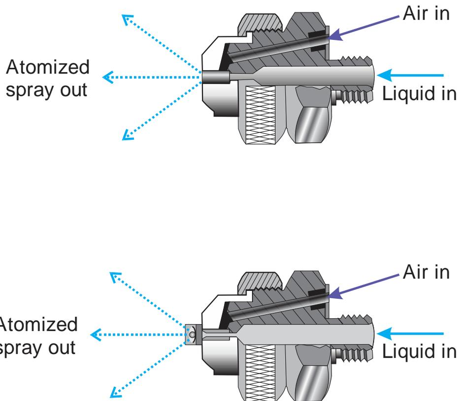
**Figure 3.5. Two styles of air atomizing nozzles. The top illustration shows a typical internal mix nozzle. The bottom illustration shows a typical external mix nozzle [adapted from SSCO 2018].**
