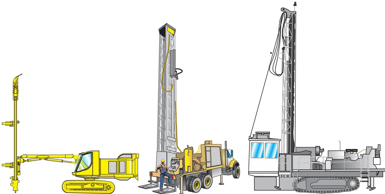
**Figure 4.1. Illustrations depicting three types of rigs. A small surface crawler drill rig is on the left, a truck-mounted drill rig is in the center, and a large track-mounted drill rig is on the right.**
