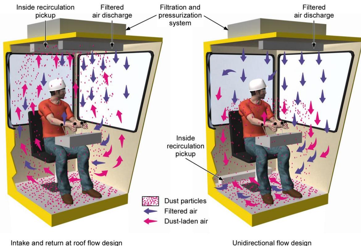
**Figure 10.18. Illustration of the airflow pattern for intake and return at the roof of a cab and a unidirectional airflow design.**
