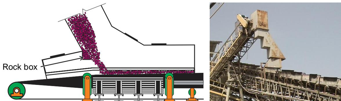
**Figure 6.6. Rock boxes used to minimize impact of falling material. The left illustration shows a rock box softening the load by reducing the drop height, with ore used as the deflection mechanism in order to reduce wear on metal parts. The right photo shows a series of rock boxes redirecting the material from one belt onto the next belt.**
