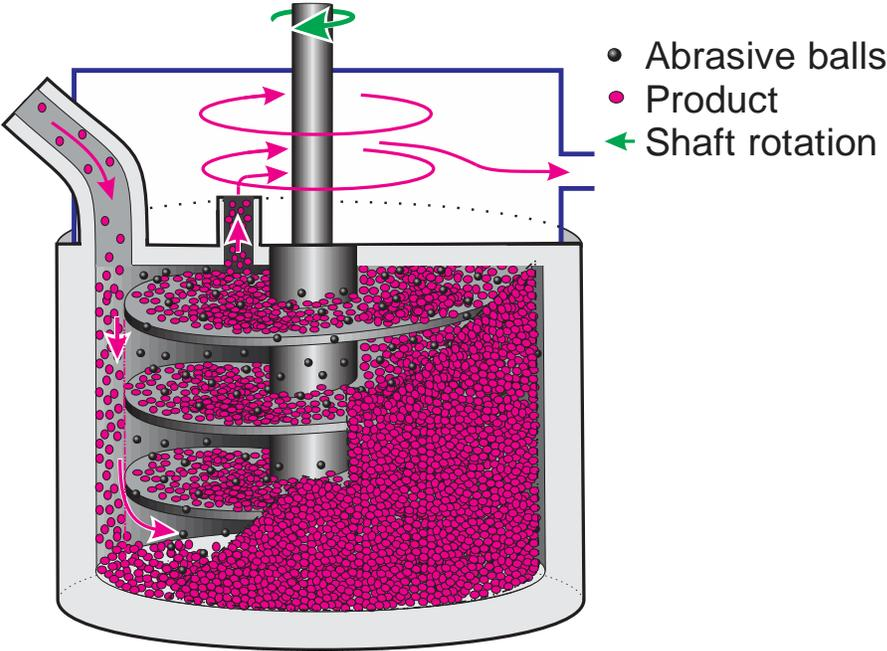
Figure 5.13. Cutaway illustration of a stirring mill.
