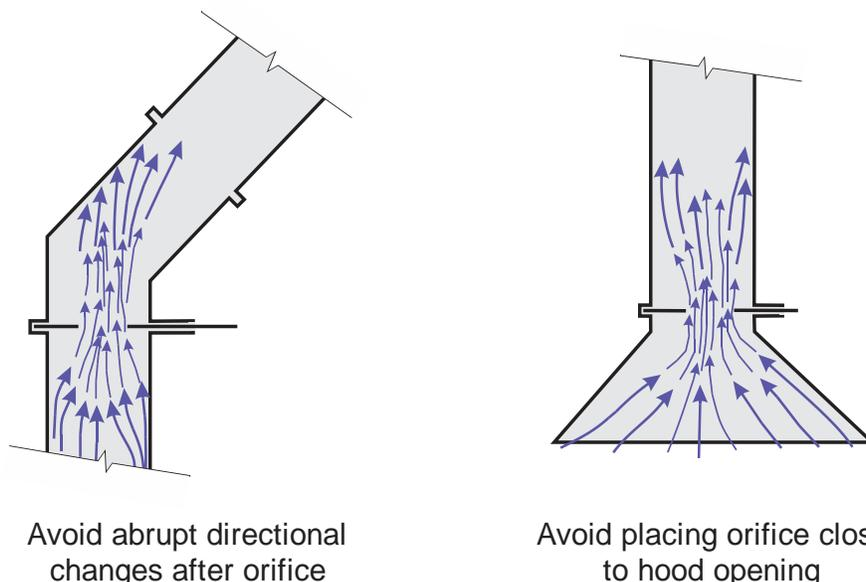
**Figure 2.13. Illustration demonstrating poor orifice plate placement.**
