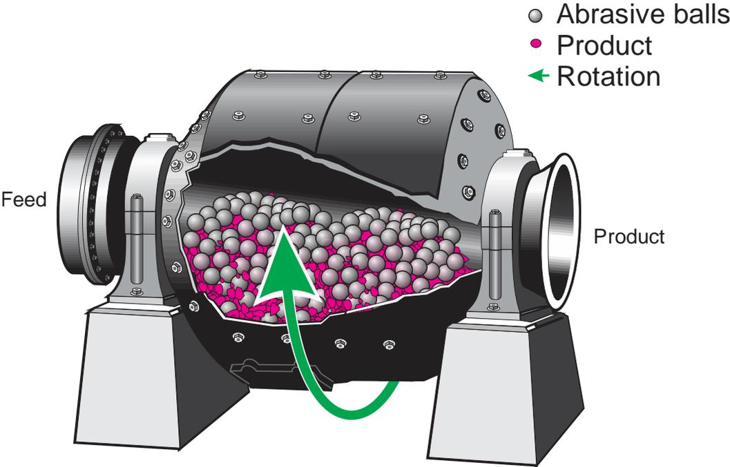
Figure 5.12. Cutaway illustration of a ball mill.
