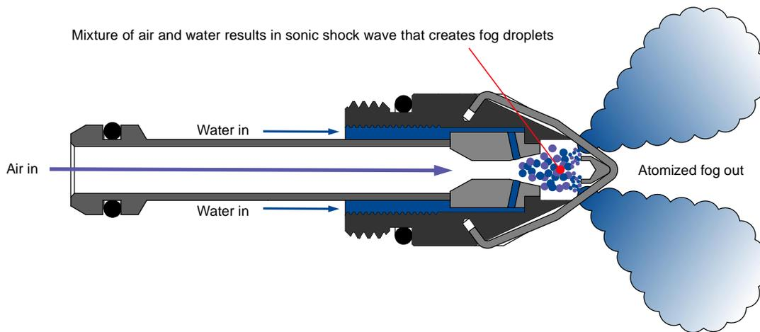
**Figure 3.13. Illustration of an ultrasonic dry fog nozzle principle of operation [adapted from Dust Solutions 2018].**
