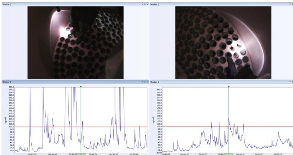
**Figure 9.1. Screenshot from the EVADE software showing video stills and respirable dust exposures for two coworkers. The video stills and graphs show respirable dust exposures for Worker 1 (left) and Worker 2 (right) while changing filter canisters inside the same local exhaust ventilation system at the same time (i.e., in the same confined space). Note that the respirable dust exposure of Worker 1, who was wearing a contaminated sweatshirt, was three times higher than that of Worker 2.**
