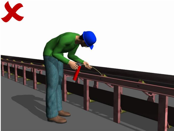
**Problem:** Without an access line, the worker has to bend to access the grease fitting and for the remaining time spent greasing.
