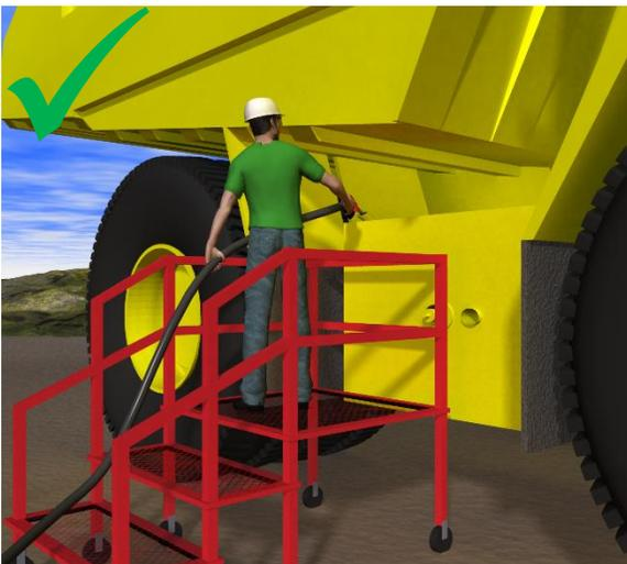
**Solution:** Add portable or permanent access platforms or step stools to areas where fueling or lubricating occurs. This encourages workers to use them while fueling or lubricating mobile equipment, such as haul trucks, at the ideal working height near waist level.
