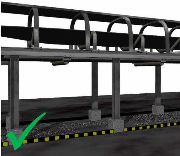
**Solution:** Add a barrier adjacent to the walkways to prevent spillage from entering walkways and causing slips. For example, a toe plate added along a conveyor and adjacent to the walkway could stop conveyor spillage from entering the walkway. If the toe plate is brightly colored and clearly marked, it helps prevent tripping when working close to or under the conveyor.
