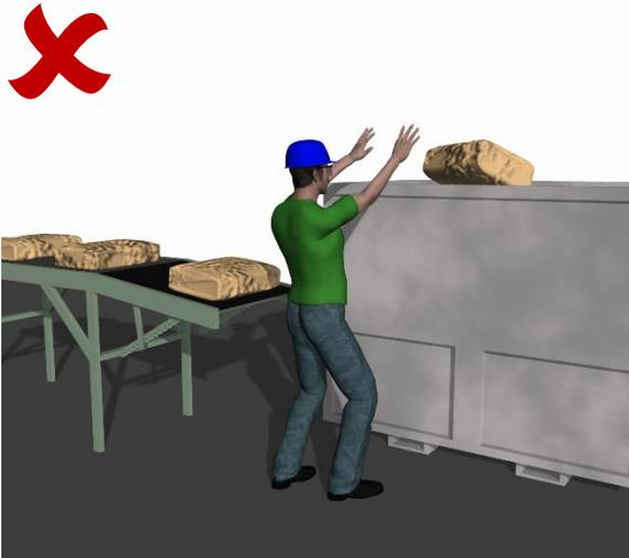
**Problem:** When scrap materials need to be moved from conveyers to dumpsters with a high lip, the material may need to be lifted at or above shoulder height and lead to musculoskeletal injuries.
