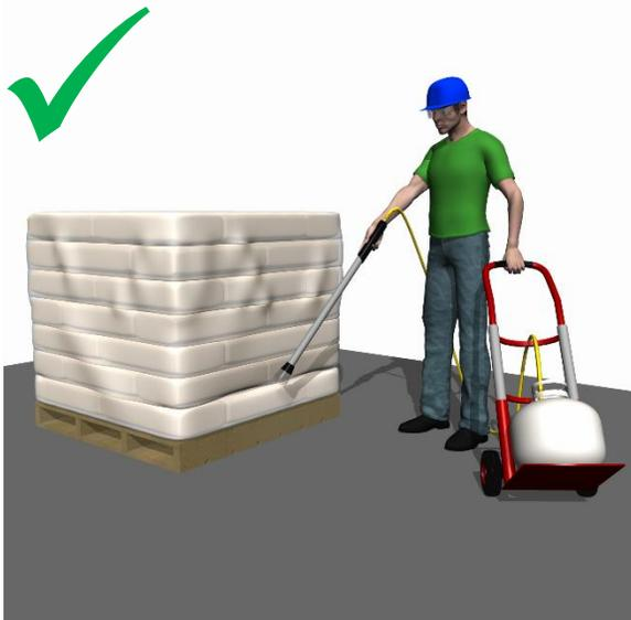
**Solution:** Supply a wheeled cart for the propane tank. This allows the worker to pull the cart instead of manually carrying the tank, which may weigh over 20 lbs.
