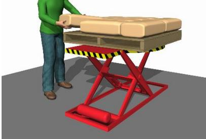
**Solution:** Provide a self-adjusting lift table to improve access and safety by ensuring workers are working near elbow height. When possible, use a rotating lift table to reduce reaching to access the differing areas on the pallet.
