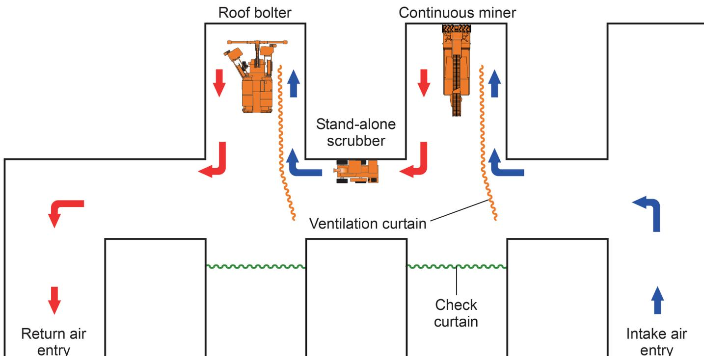
Figure 2. Underground mine application of the DS cleaning air downwind of the continuous miner and upwind of the roof bolter.
