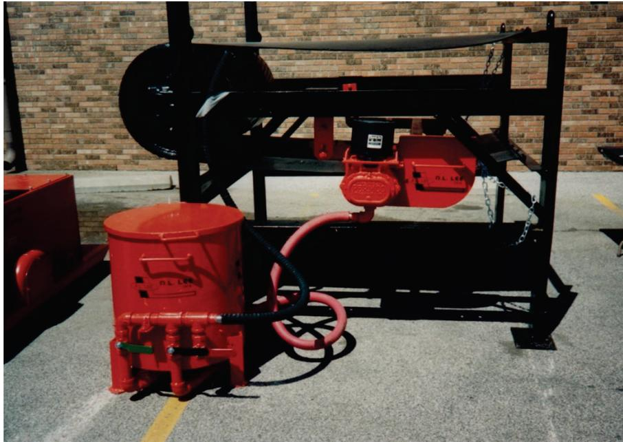
**Figure 9. Photograph of a belt-powered Master II Trickle Duster.**
