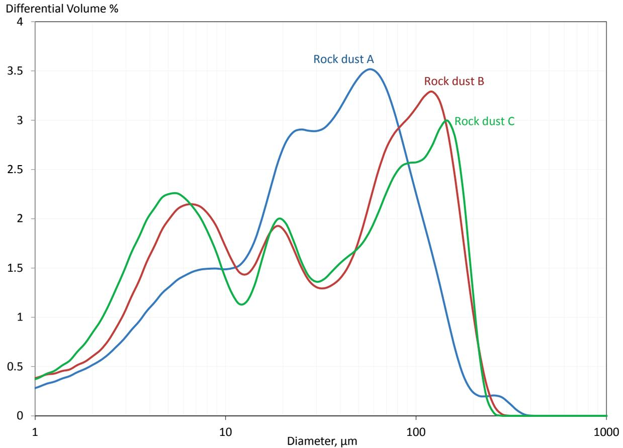
**Figure 17. The differential volumes of the three rock dusts used during the wet rock dusting applications.**
