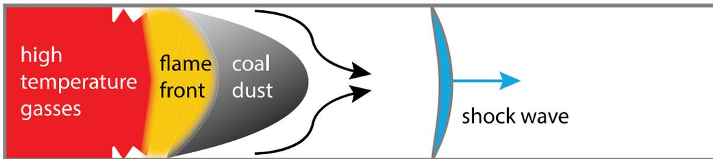
**Figure 2. The flame front appears behind the shock wave.**
