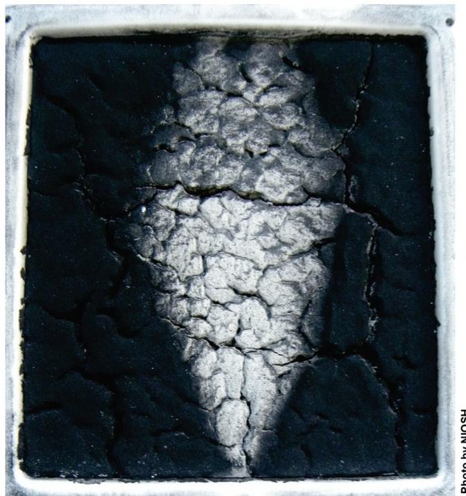
**Figure 4. An explosive layer of float coal dust covers a tray filled with rock dust; both materials were subjected to moisture and then dried. A pulse of air applied across the top of the tray removed only the layer of still dispersible float coal dust but not the caked rock dust.**
