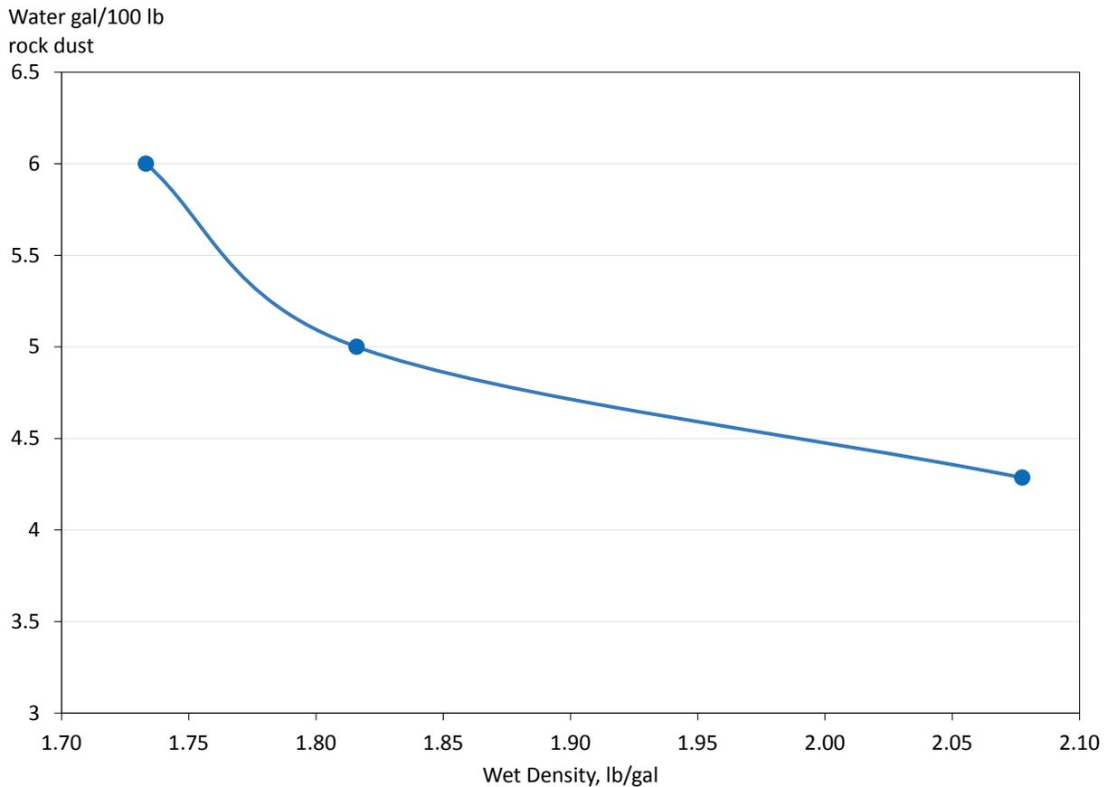
**Figure 15. Water content relationship to wet rock dust density for Rock Dust C.**
