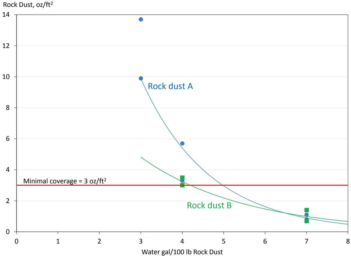
**Figure 13. Ounces of dry rock dust per square foot with respect to the wet rock dust slurry mix.**
