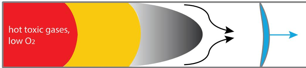
**Figure 3. The cycle continues with the shock wave lifting coal dust and the lagging flame front igniting and propagating the explosion.**
