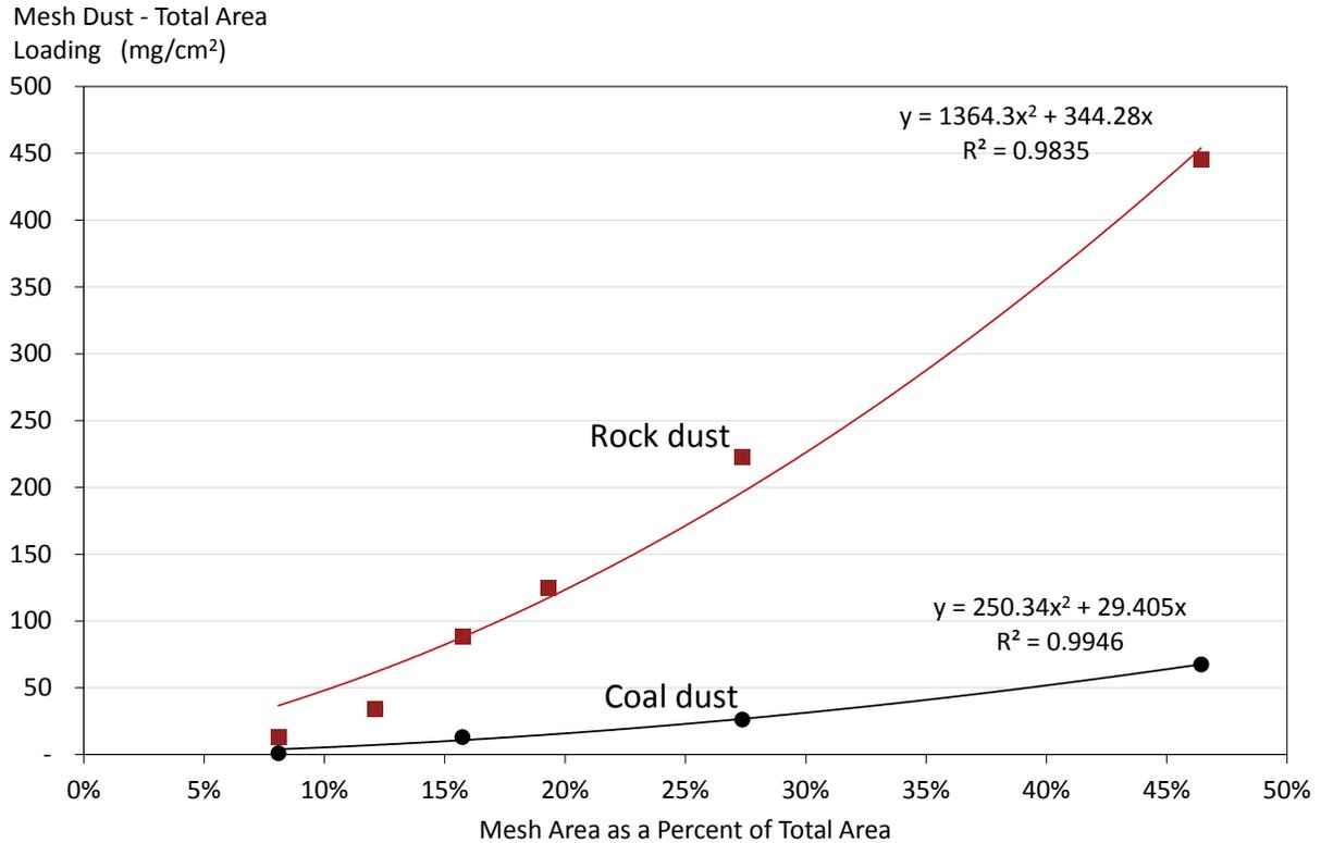
**Figure 11. Mesh-carrying capacity of rock dust and coal dust.**
