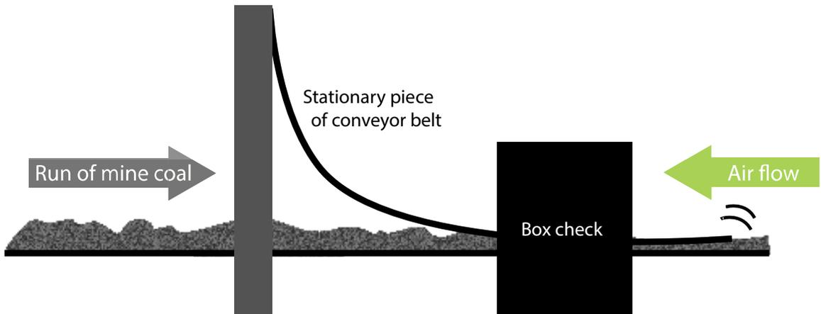
Figure 8. Conveyor belt traveling through a box check with a stationary section of conveyor belt to sandwich run of mine coal between the mine conveyor belt and the stationary section of belt, reducing coal spillage at that location.
