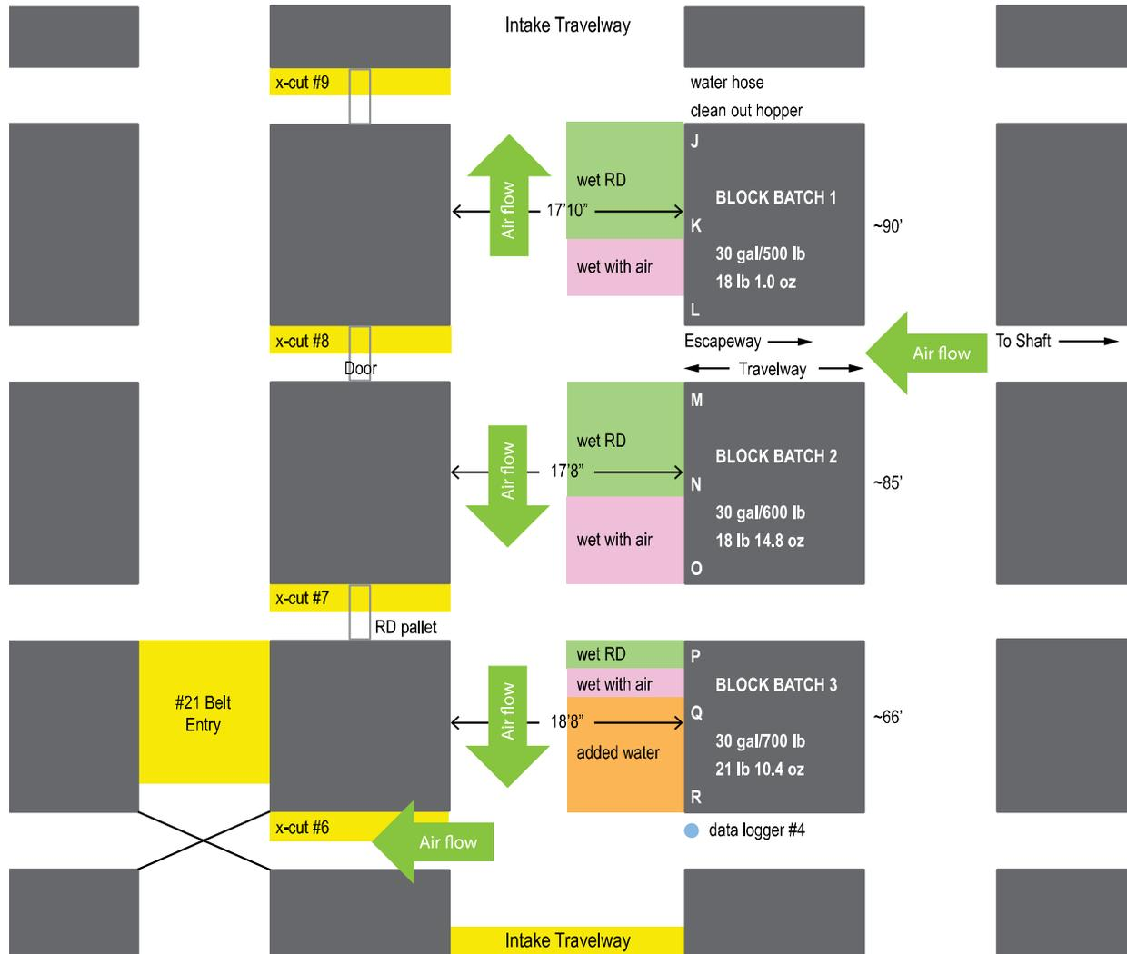
**Figure 14. Wet rock dust test area and data in the West Virginia mine.**
