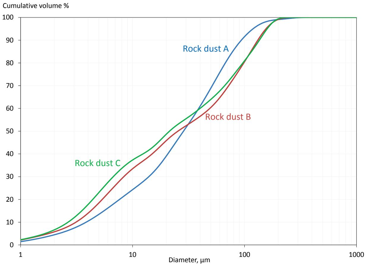
**Figure 16. The cumulative particle size distribution of the rock dusts used during the wet rock dusting applications.**
