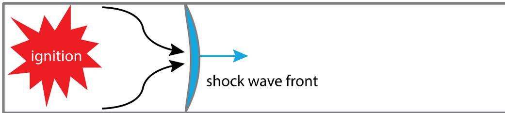
**Figure 1. Beginning stage of a propagating coal dust explosion.**
