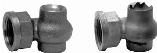
**Figure 2.15. Nozzle erosion—new versus used [Schick 2006].**
