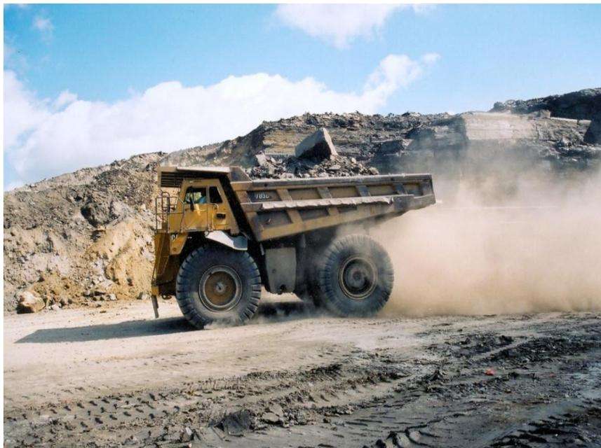
**Figure 10.1. Example of haul road dust from a typical mine haul truck.**
