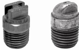
**Figure 2.19. Nozzle damage—new versus used [SSCO 2003].**
