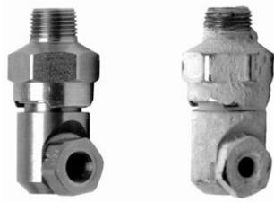
**Figure 2.17. Nozzle caking—new versus used [Schick 2006].**
