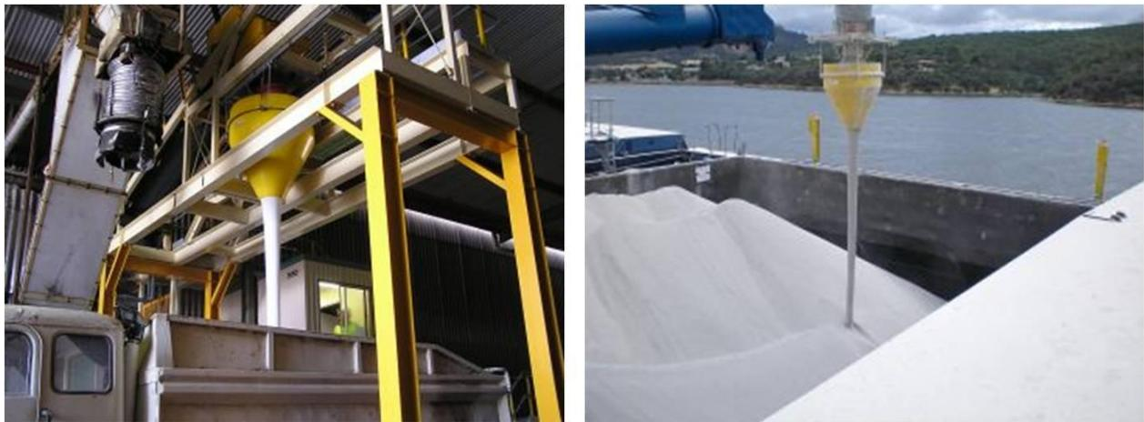
**Figure 7.6. Dust Suppression Hopper creating a solid stream of material during loading to reduce dust liberation.**
