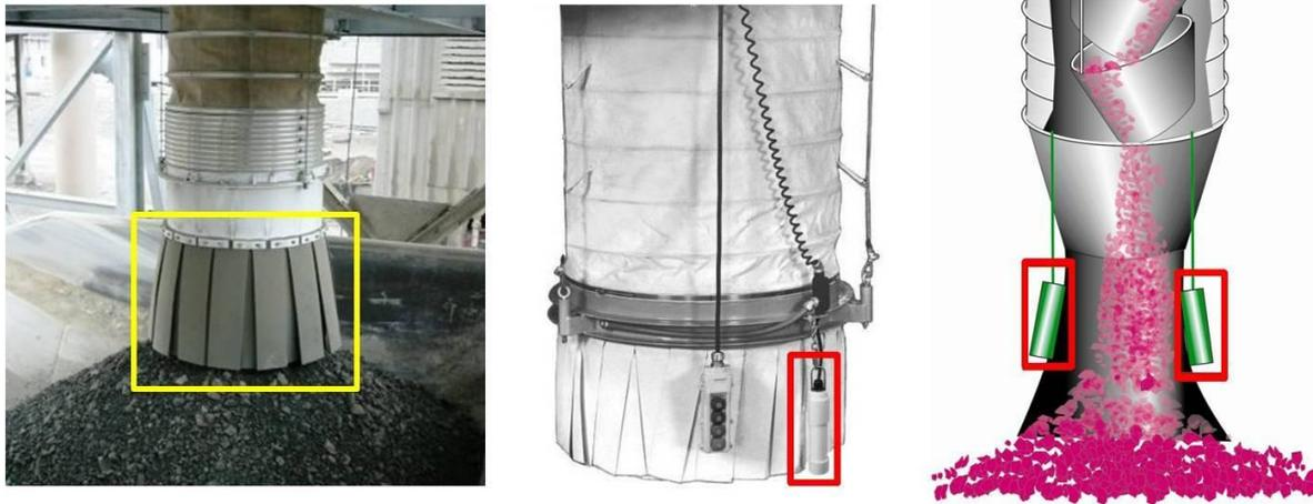
**Figure 7.4. Skirt (in yellow box) and tilt sensors (in red boxes) installed on the discharge end of loading spouts to help reduce dust emissions.**
