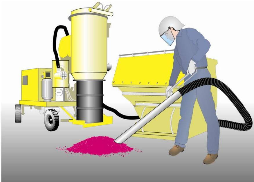
**Figure 8.6. Portable system used to perform vacuuming.**
