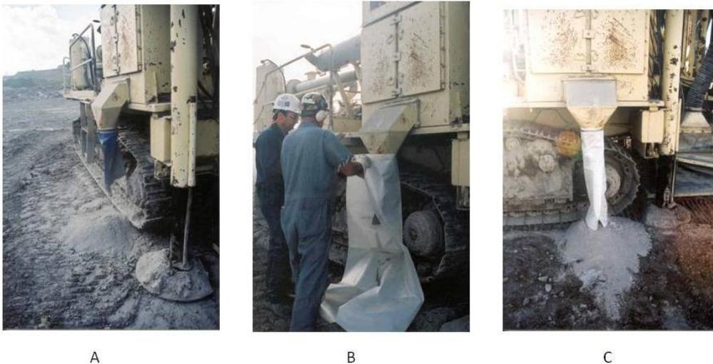
**Figure 3.13. Dust collector dump point prior to shroud installation (A). Two men installing the shroud onto the dust collector dump point (B). The dust collector dump point after installation of the shroud (C).**
