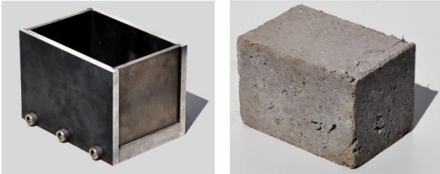
Figure 2. Partial beam box mold and test specimen.
