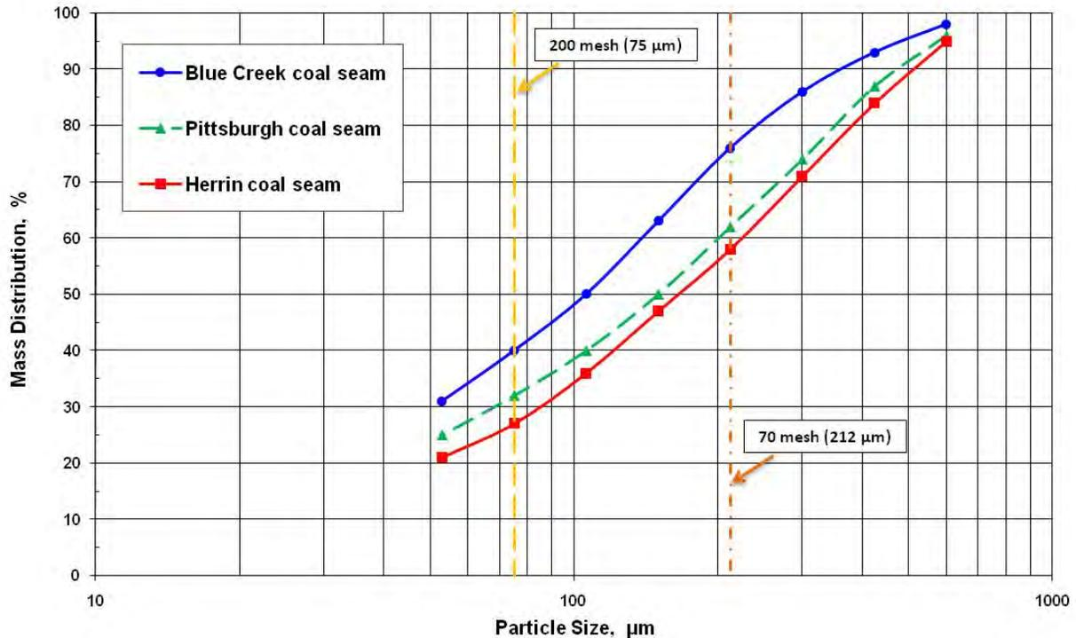
Figure 10. Coal particle size by coal seam.
