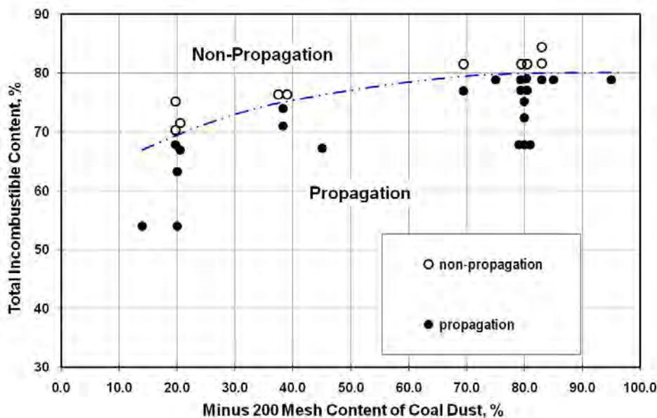
Figure 11. Effect of particle size of coal dust on the explosibility of Pittsburgh seam bituminous coal as tested within LLEM.
