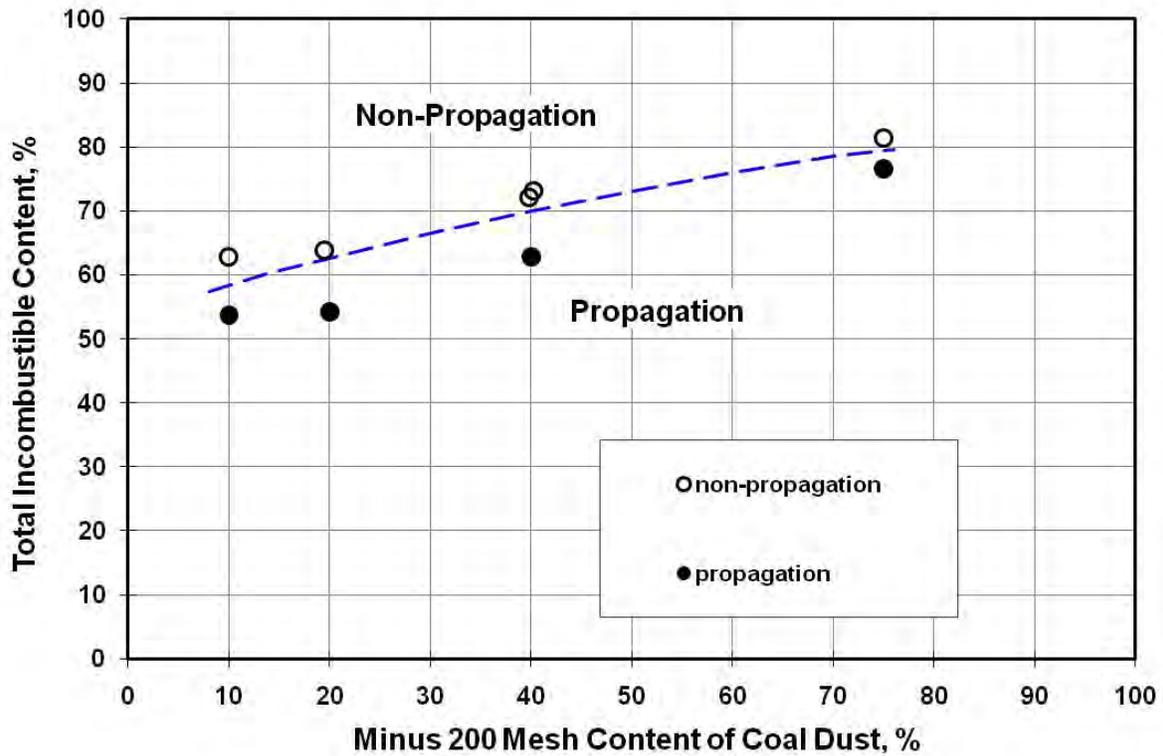
Figure 1. Effect of particle size of coal dust on the explosibility of Pittsburgh seam bituminous coal as tested within BEM.
