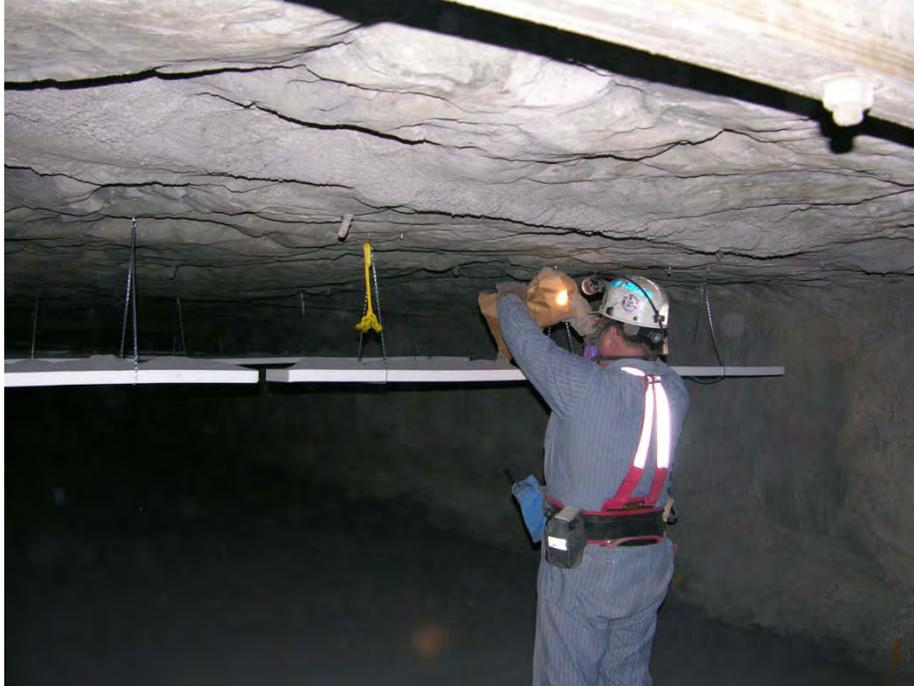
**Figure 7. Placing coal and rock dust mixture on shelves in the LLEM.**
