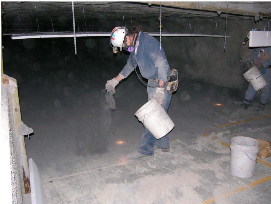
**Figure 8. Distributing test dust mixture at the LLEM.**
