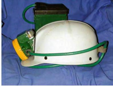
**Figure 71. Cap lamp-mounted methane monitor.**
