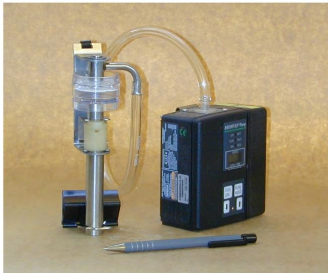
Figure 2-1. Gravimetric sampling pump, cyclone and filter cassette.
