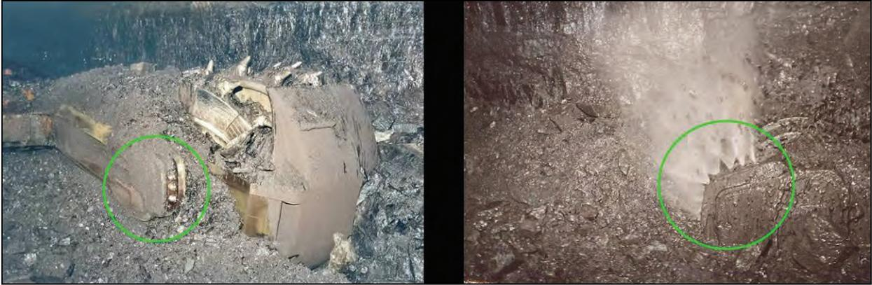
Figure 3-13.—Crescent sprays located on shearer ranging arm.
