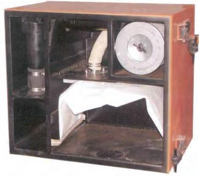
Figure 4-14.—Dust collector box with collector bag installed.
