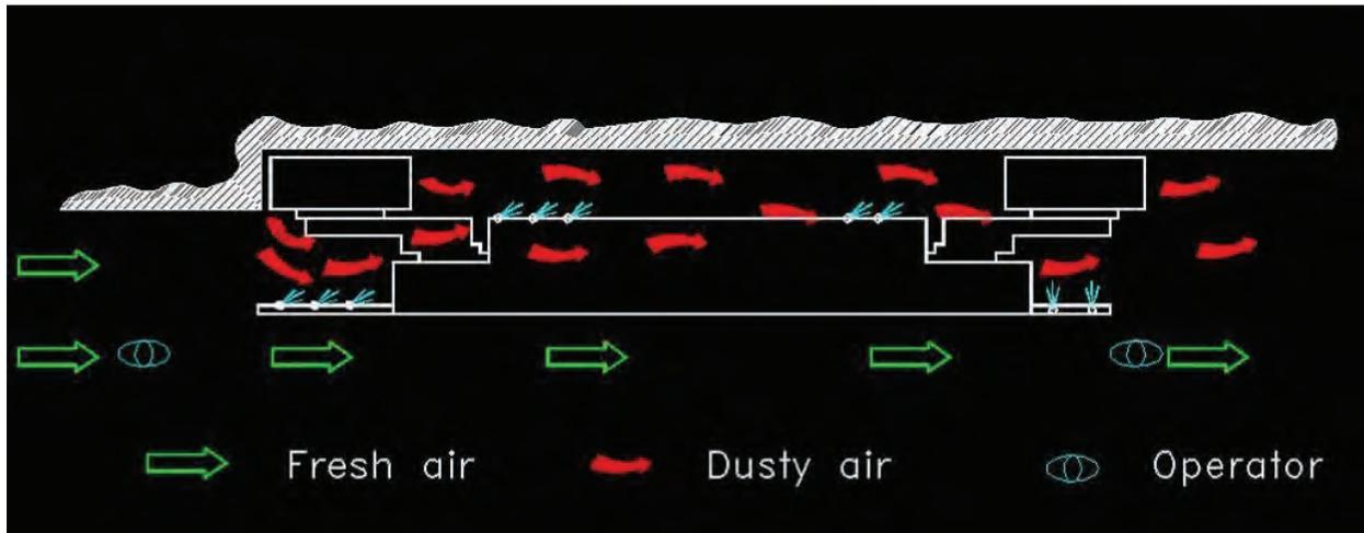
Figure 3-7.—Shearer-cleaver directional spray system.
