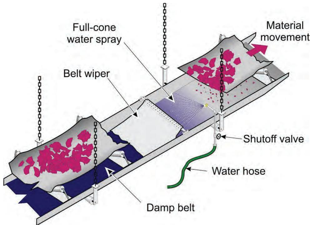
Figure 3-2.—Water sprays and belt wiper used to reduce dust from the nonconveying side of the belt as it returns.
