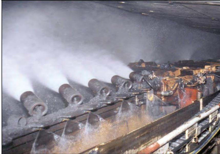
**Figure 3-8.—Venturi sprays mounted on headgate splitter arm.**
