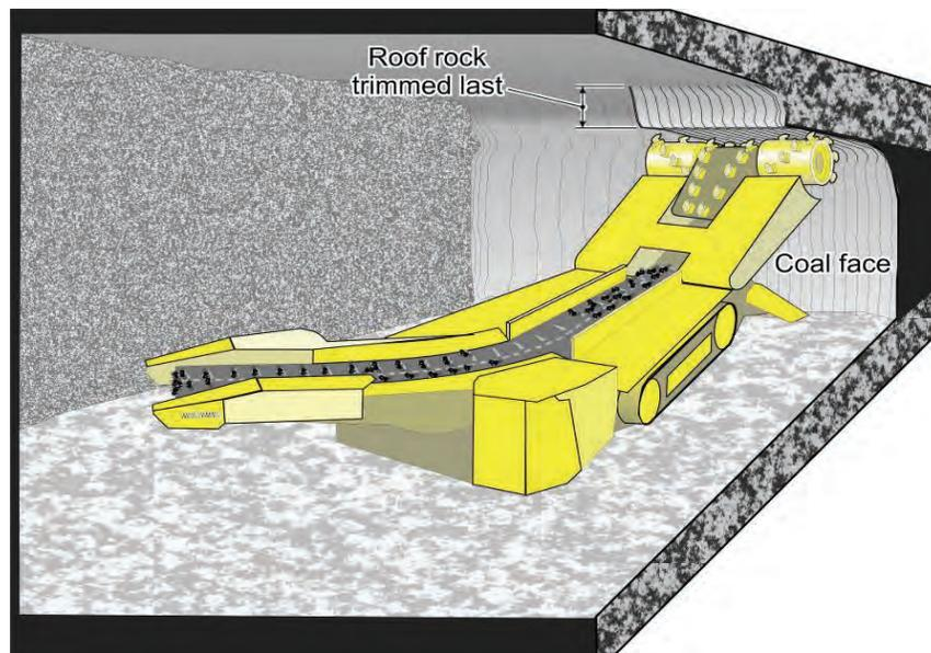
Figure 4-11.—Modified cutting cycle can lower dust generation.
