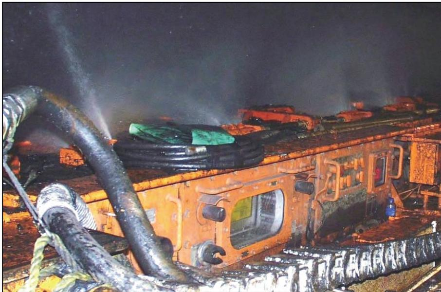
**Figure 3-10.—Directional sprays mounted on face side of shearer body.**
