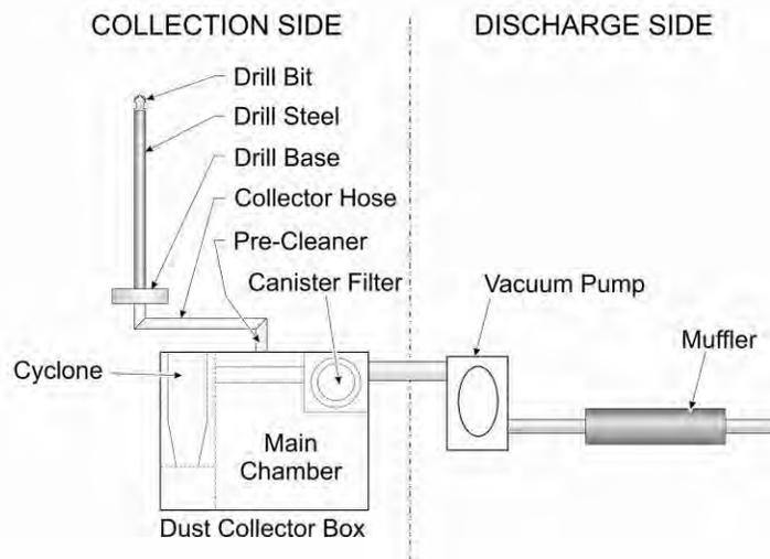
Figure 4-15.—Schematic of roof bolter dust collector components.
