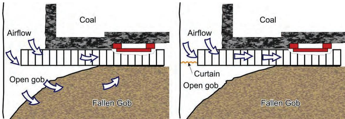
Figure 3-5.—Gob curtain increases airflow down the face.
