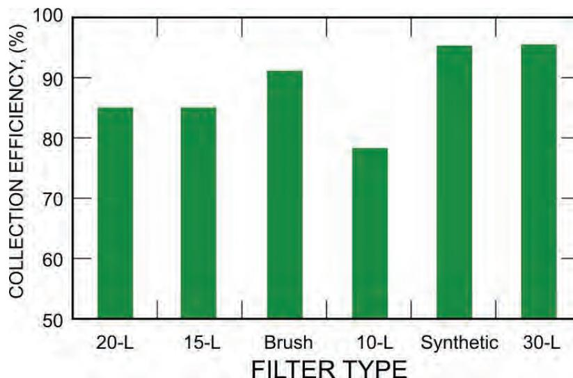
Figure 4-9.—Dust collection efficiency of scrubber filter panels.
