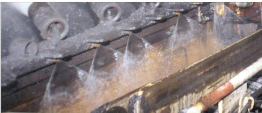
**Figure 3-9.—Headgate splitter arm with flat-fan sprays mounted on gob side of belting.**
