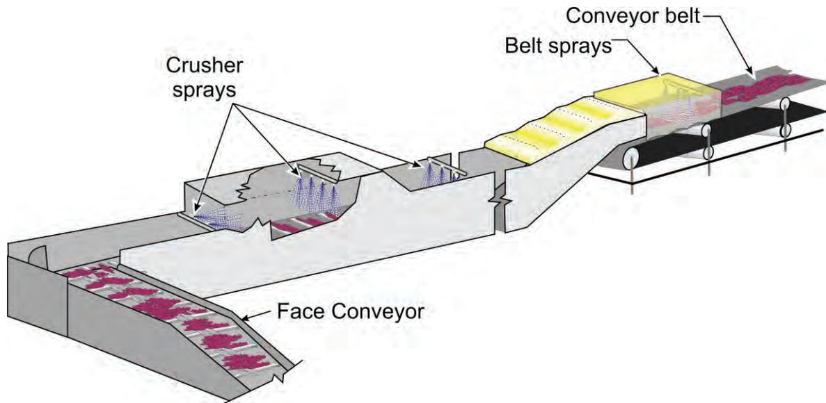
Figure 3-3.—Enclosed stageloader/crusher and location of water sprays.
