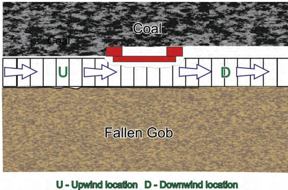
**Figure 2-5.—Mobile sampling used to quantify shearer dust.**
