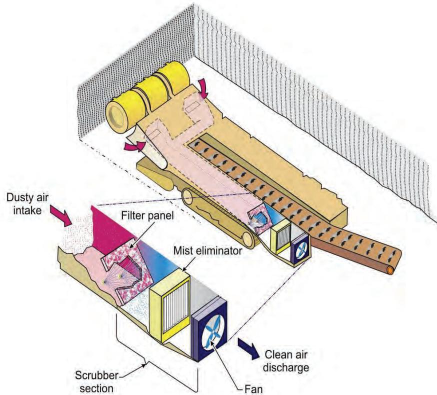
Figure 4-6.—Components and design of a flooded-bed scrubber.
