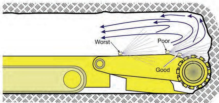
**Figure 4-3.—Spray location impact on dust rollback.**
