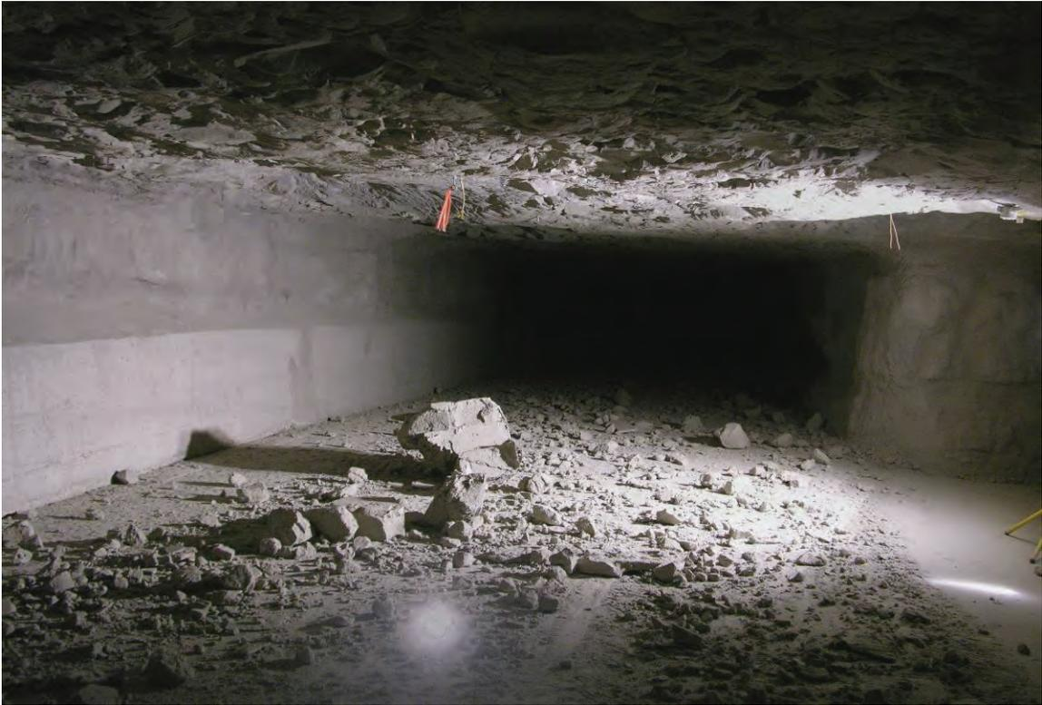
**Figure 21.—Debris after Test 2 (LLEM #502) looking outby from X-6 location.**
