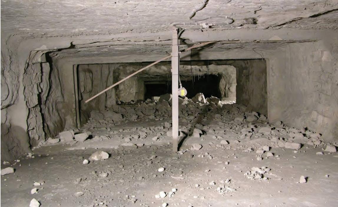
**Figure 42.—Debris from X-3 seal after Test 5 (LLEM #505) looking into X-3 toward B-drift.**
