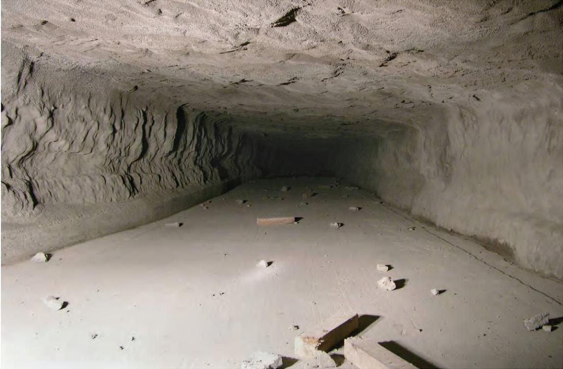
**Figure 75.—Debris in C-drift after Test 6 (LLEM #506) looking outby from ~1,240 ft.**
