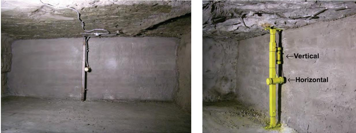
Figure 3.—Front and side views of pressure transducers in front of seals.
