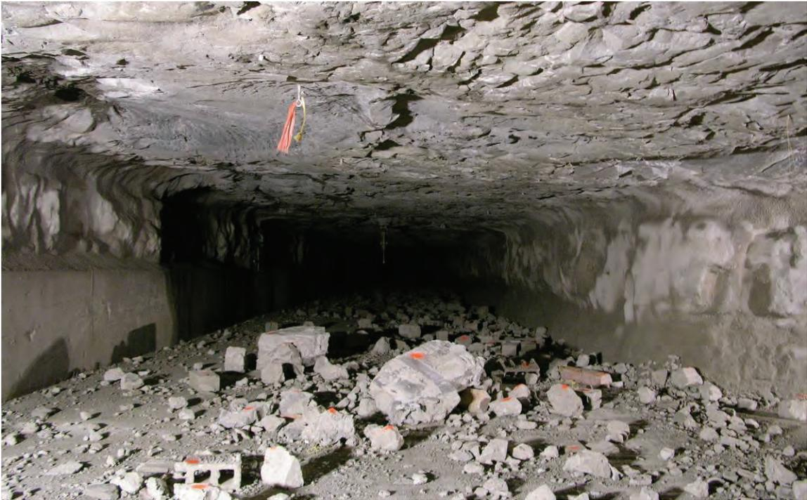
**Figure 48.—Debris in C-drift after Test 5 (LLEM #505) looking outby from X-6 at 547 ft.**
