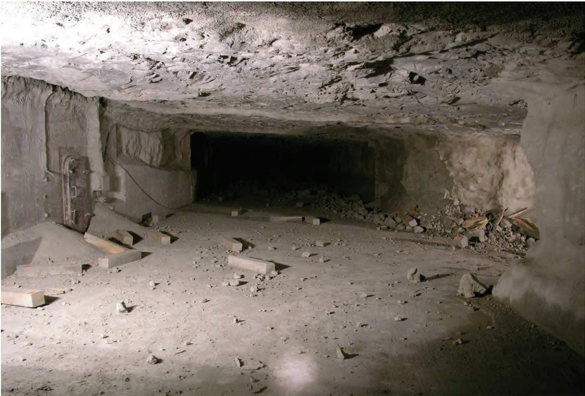
Figure 46.—Debris in C-drift after Test 5 (LLEM #505) looking outby toward X-4 (right side of photo) at 355 ft.
