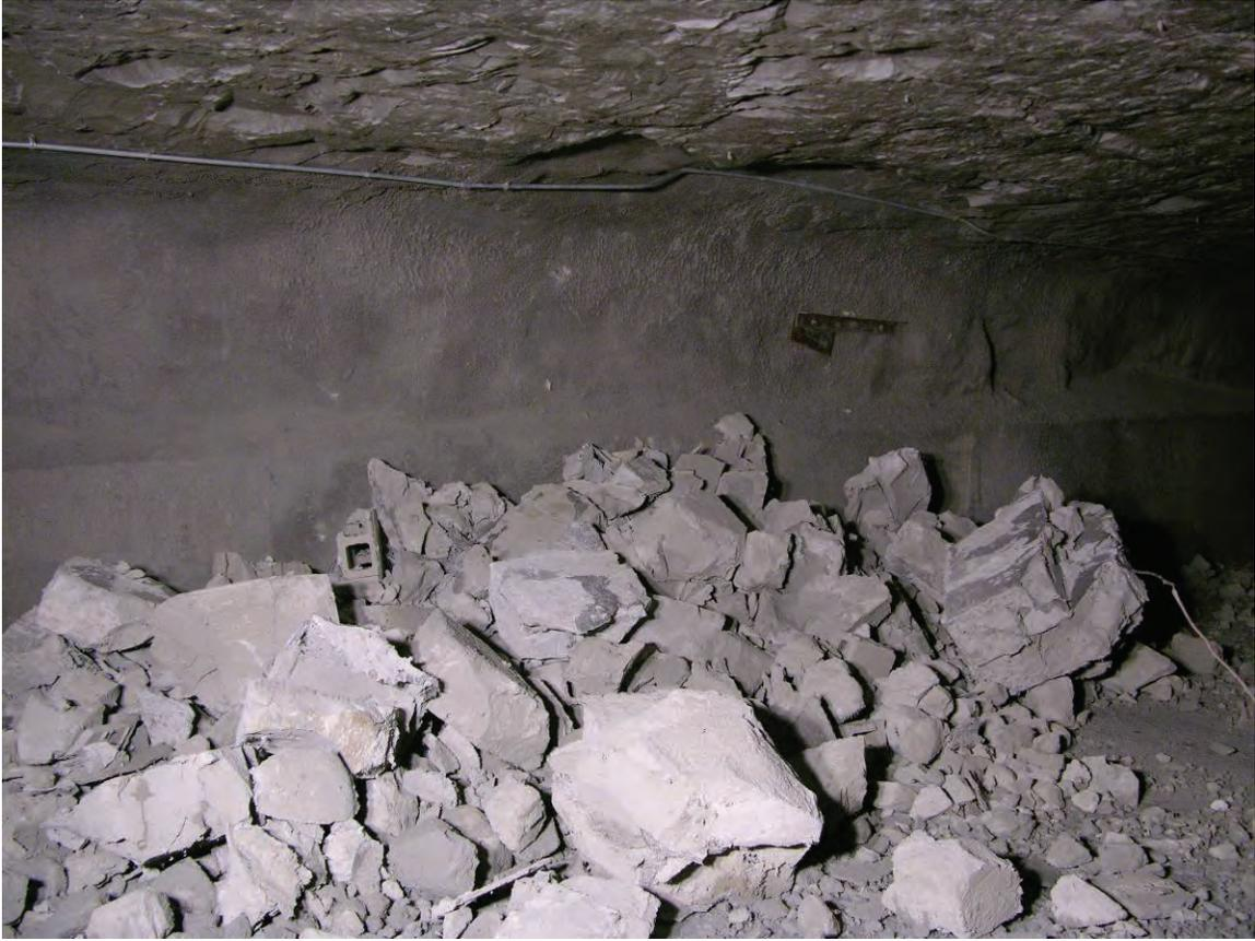
**Figure 44.—Debris from the X-3 seal and stopping piled against the far wall of A-drift after Test 5 (LLEM #505).**
