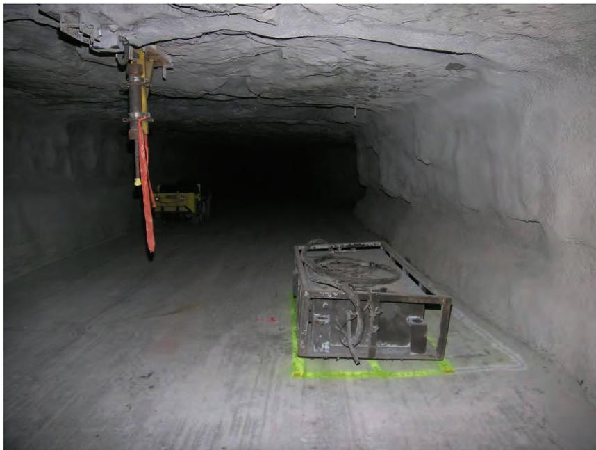
**Figure 11.—Battery charger located at ~602 ft in C-drift.**
