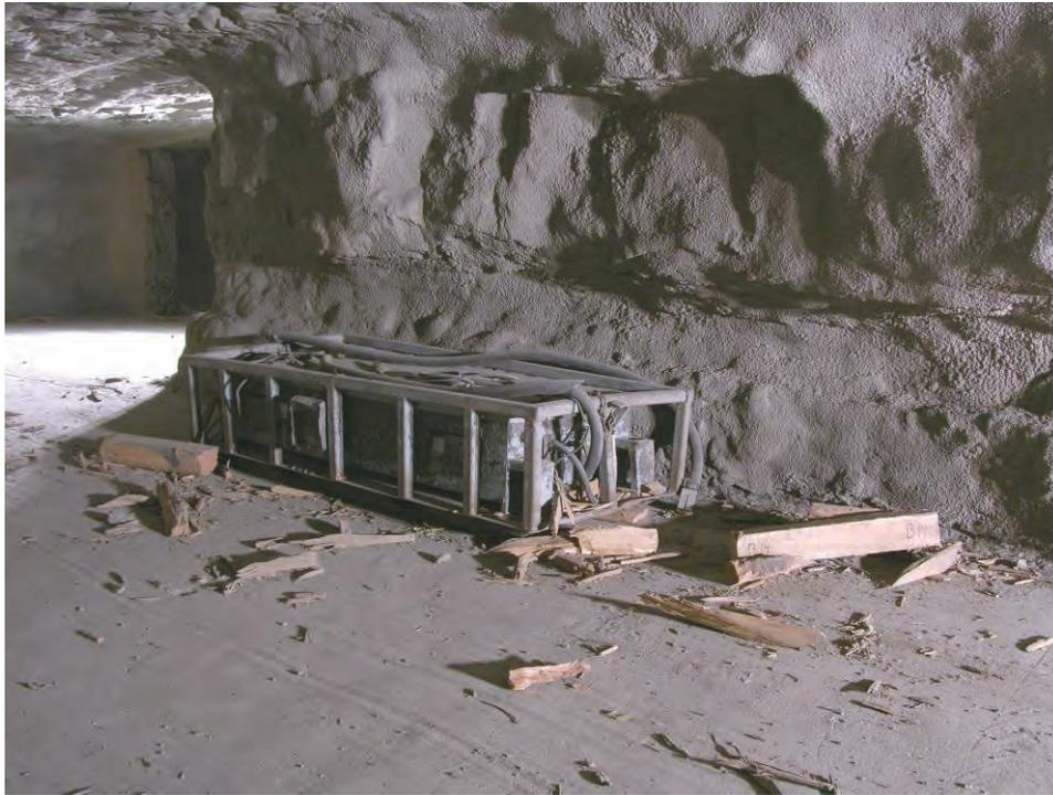
**Figure 12.—Battery charger and debris from the wood cribs near X-7 after Test 1 (LLEM #501).**
