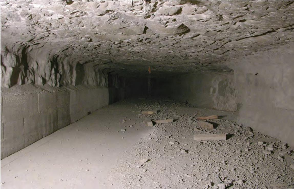
**Figure 68.—Debris in C-drift after Test 6 (LLEM #506) looking outby from ~500 ft.**
