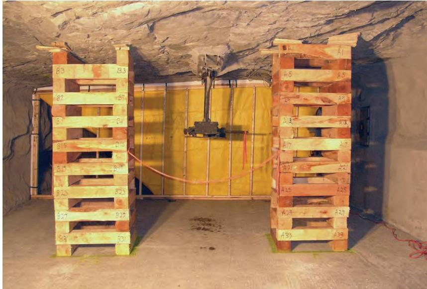
**Figure 10.—Wood cribs at 312 ft looking inby in C-drift before Test 1 (LLEM #501).**
