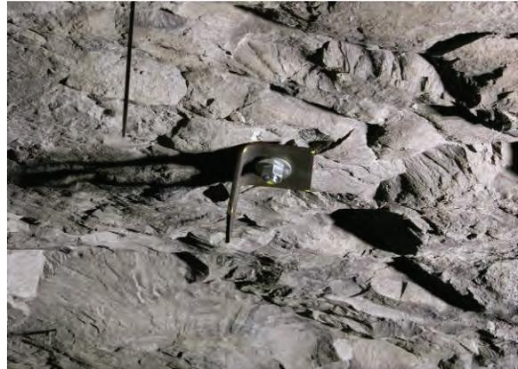
Figure 5.—Roof plates and belt hanger at 134 ft from the face.
