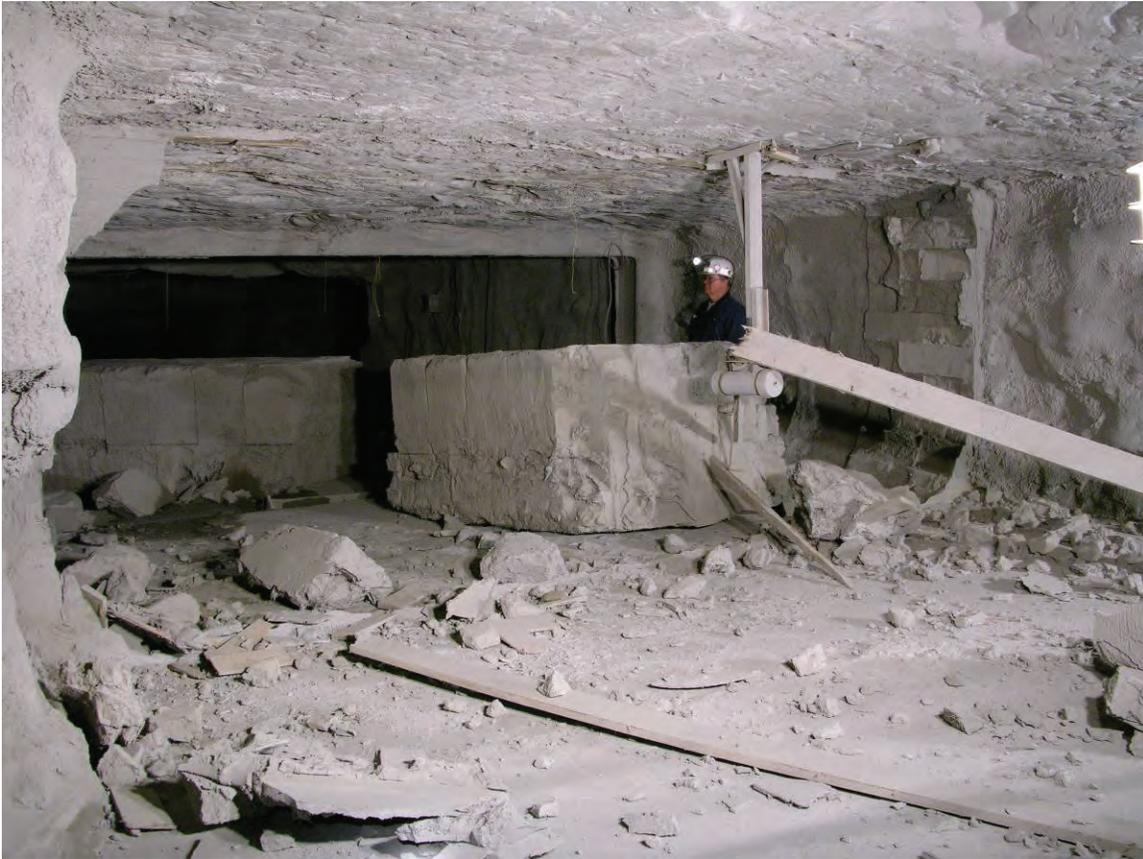
**Figure 18.—Remains of X-3 seal viewed from C-drift after Test 2 (LLEM #502).**
