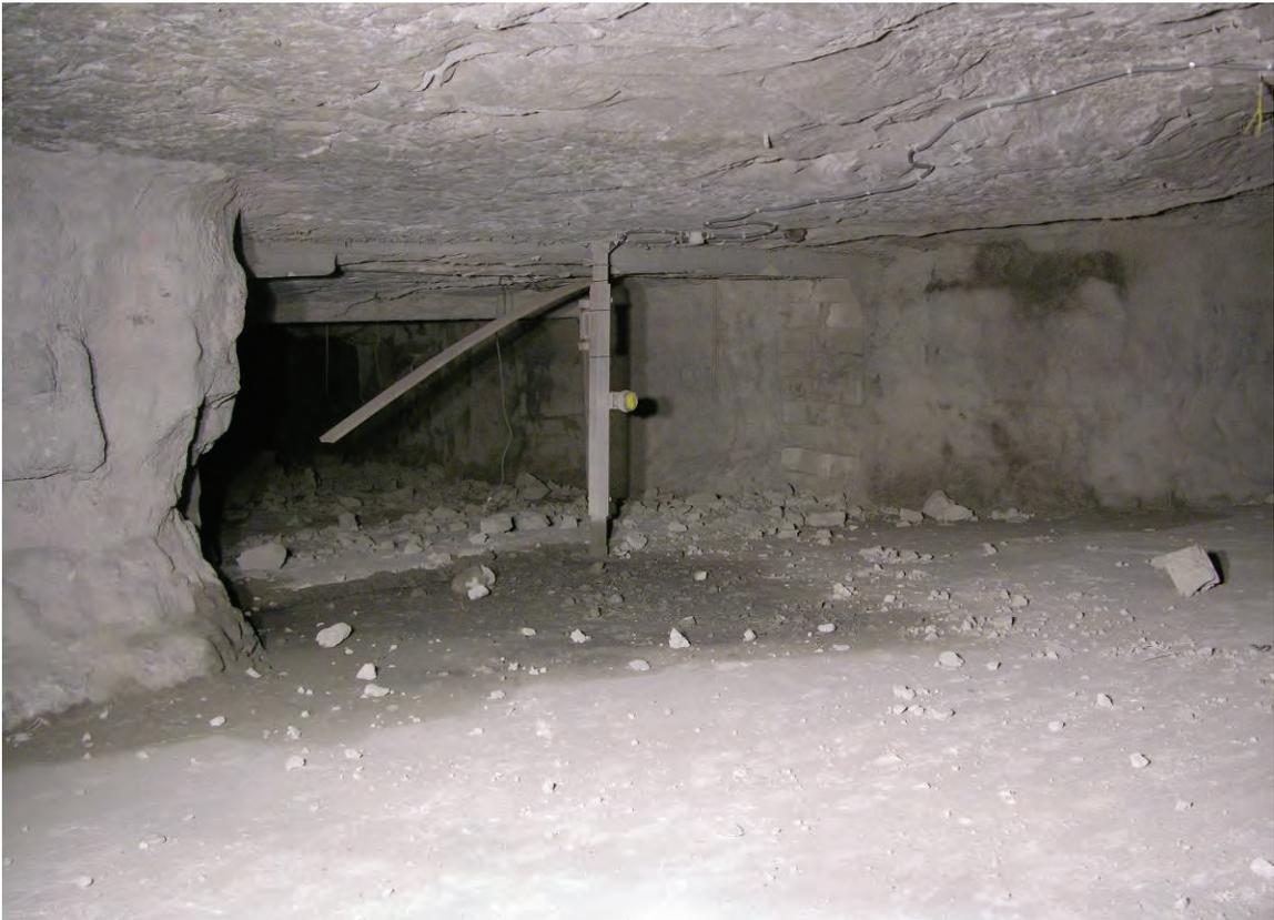
**Figure 41.—Debris from X-3 seal after Test 5 (LLEM #505) viewed from C-drift.**
