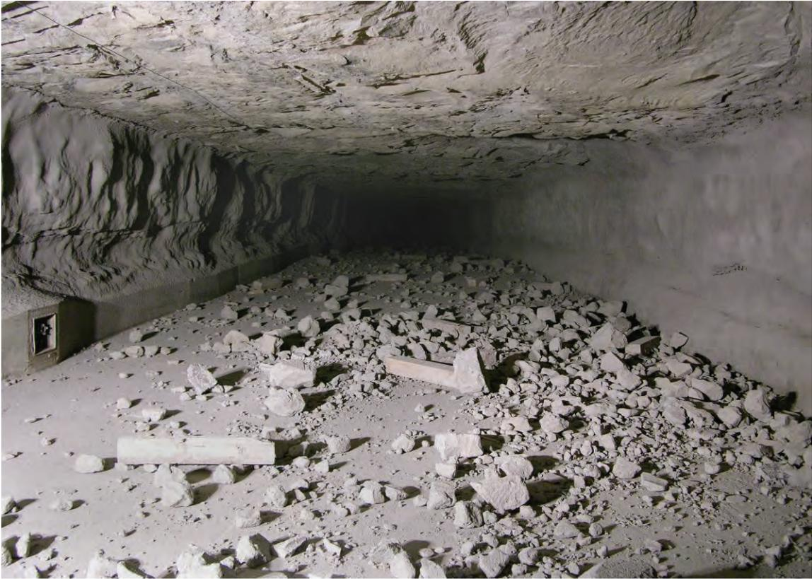
Figure 73.—Debris after Test 6 (LLEM #506) looking outby from ~1,050 ft.
