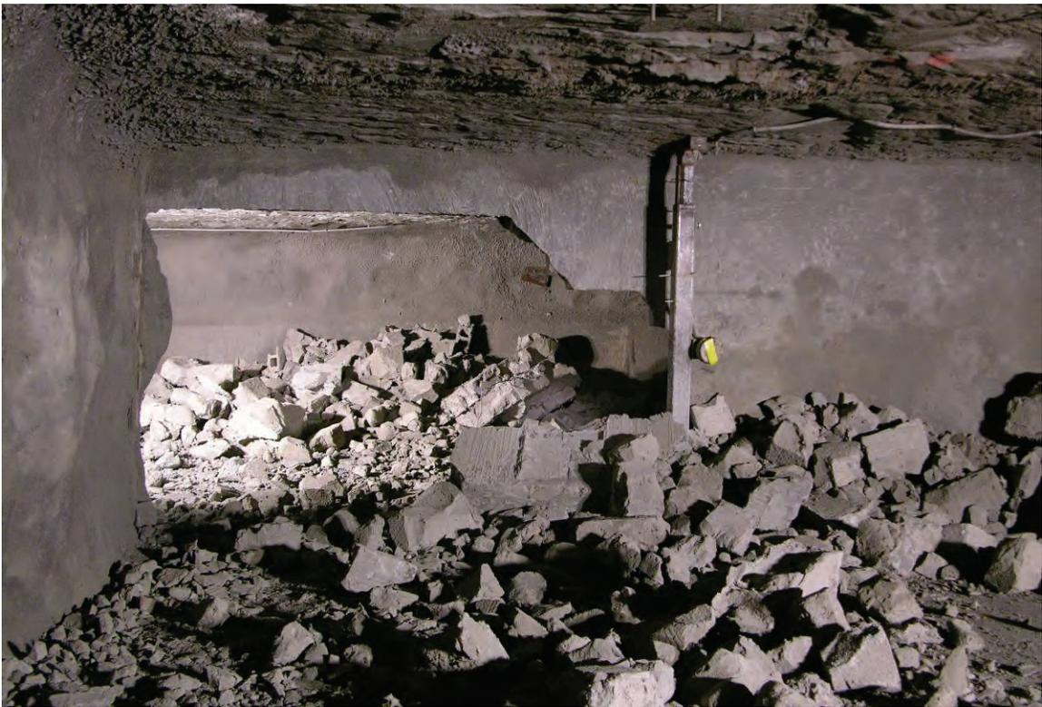
**Figure 43.—Debris from the X-3 seal at the X-3 stopping location after Test 5 (LLEM #505).**
