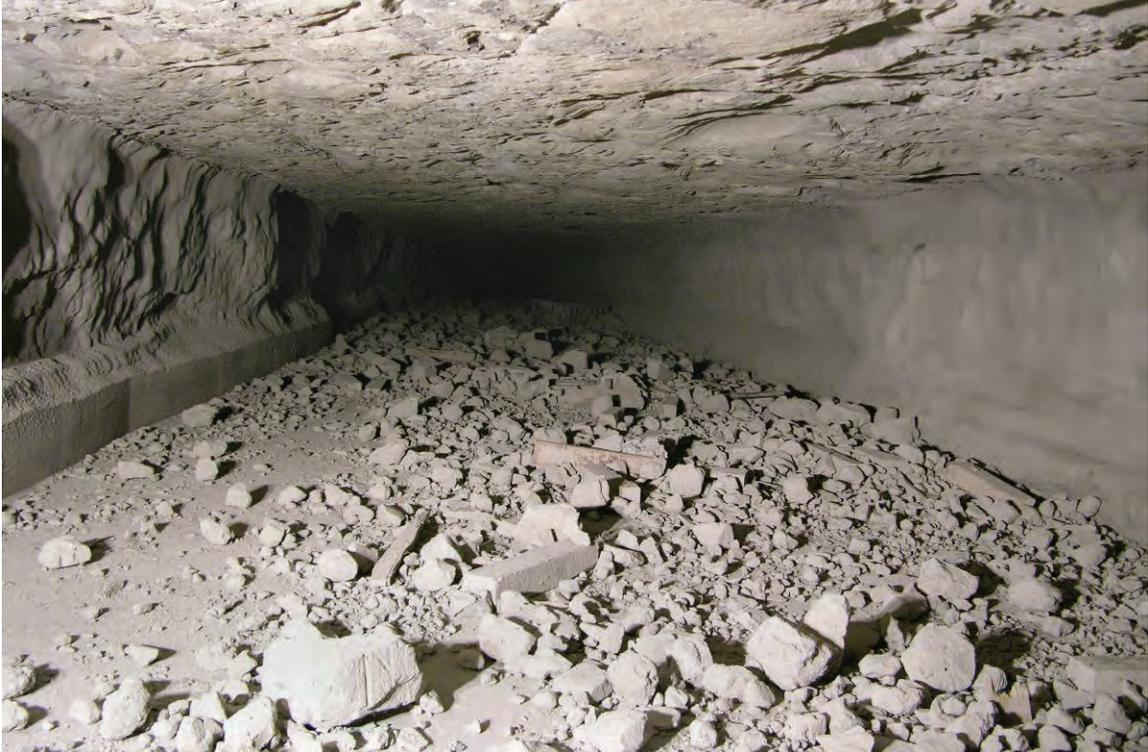
**Figure 72.—Debris after Test 6 (LLEM #506) looking outby from ~950 ft.**
