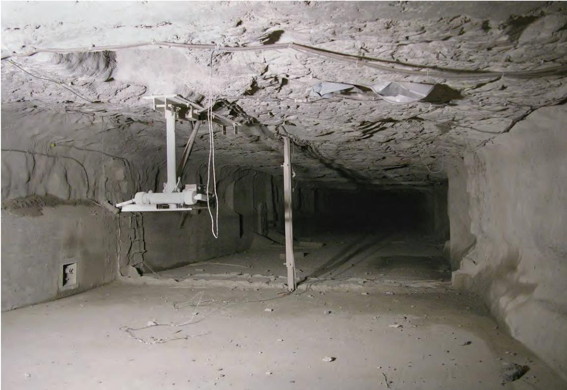
**Figure 65.—Postexplosion view in C-drift looking outby toward original seal location at 320 ft after Test 6 (LLEM #506).**
