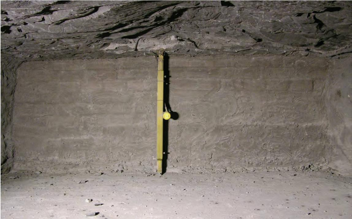
**Figure 40.—Seal in X-2 that survived Test 5 (LLEM #505).**
