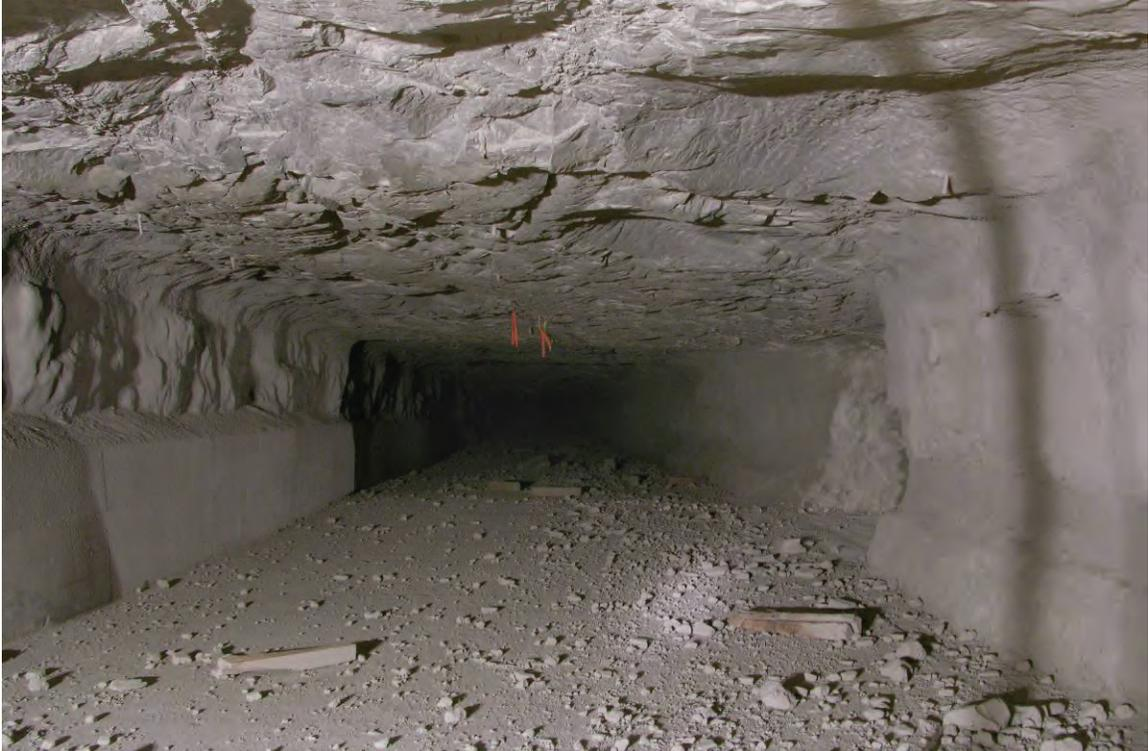
**Figure 69.—Debris in C-drift after Test 6 (LLEM #506) looking outby from ~600 ft.**
