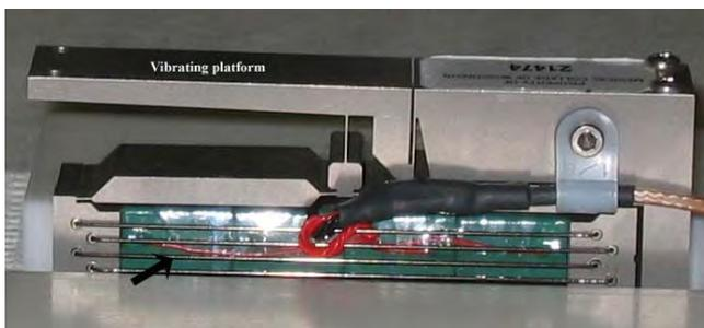
**Figure 1.—The MRI-compatible flextensional piezoelectric actuator is constructed of titanium and sheets of piezoelectric material (black arrow) that bend in response to applied voltage to cause vertical translation of the lever arm platform.**
