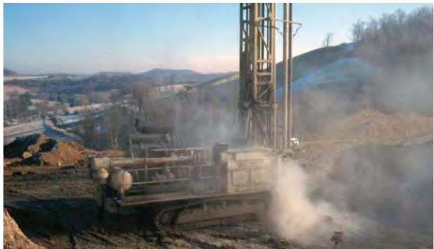
**Figure 1.** Rock drilling without appropriate dust control.
