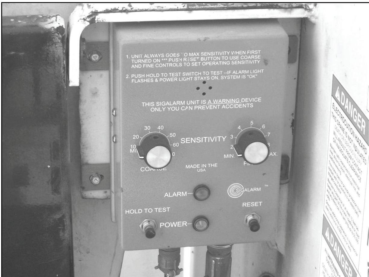
Figure 1.—SIGALARM Model 210 control unit.
