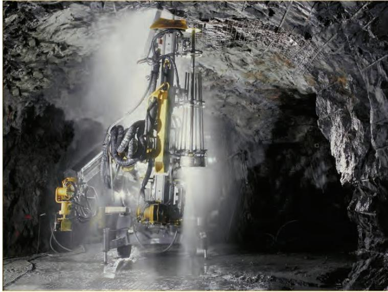
Figure 10 - Drill used to install rock reinforcement.
