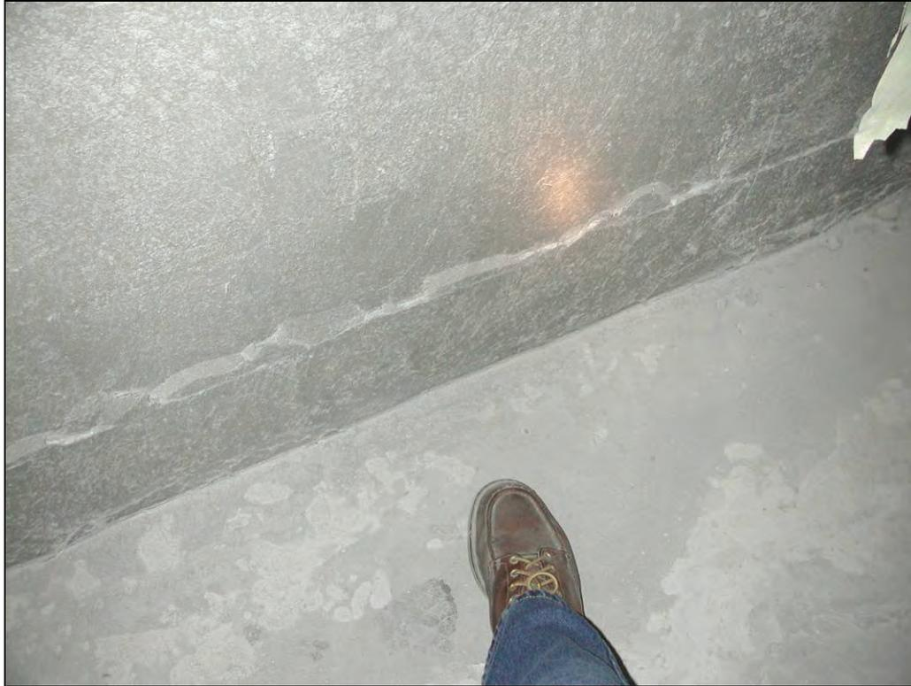
**Figure 70.—Displacement of the second block course at the X-4 dry-stacked solid-concrete-block stopping after LLEM test #459, viewed from C-drift.**
