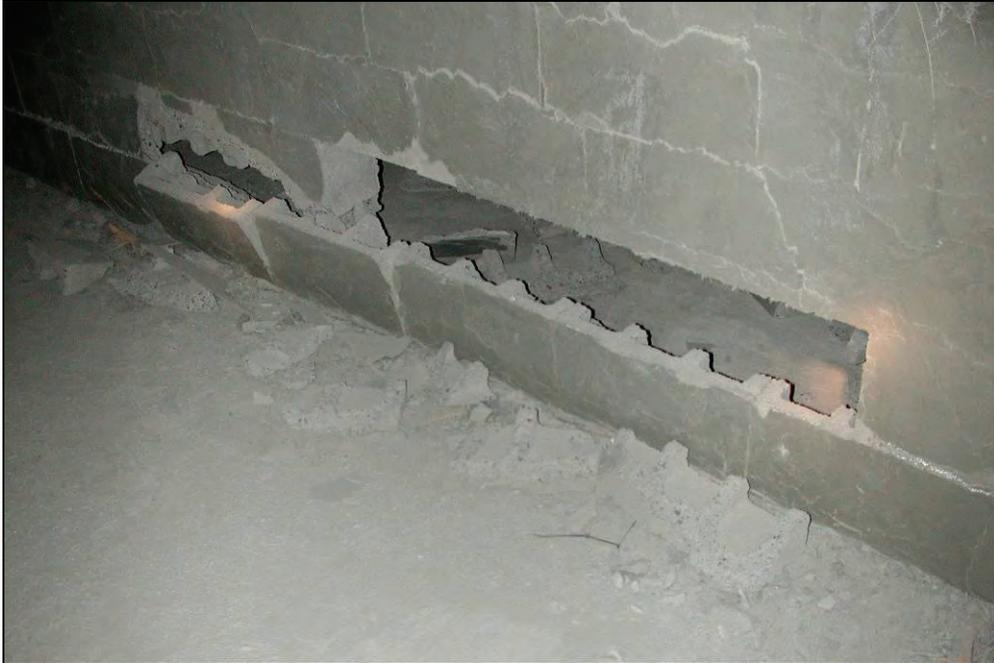
**Figure 47.—Closeup of C-drift side X-6 dry-stacked hollow-core concrete block stopping after test #430, showing missing and damaged blocks.**
