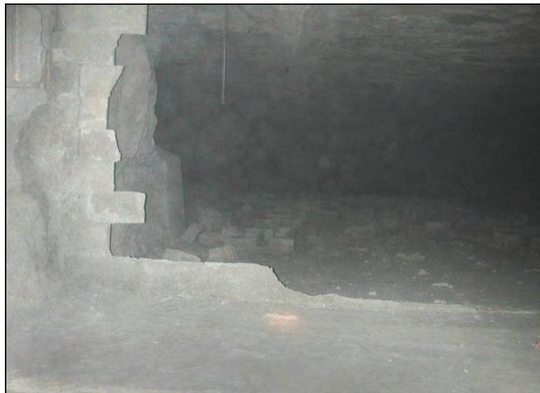
Figure 72.—Debris from the dry-stacked solid-concrete-block stopping and remaining blocks on the outby rib line in X-4 after LLEM test #462, viewed from C-drift.
