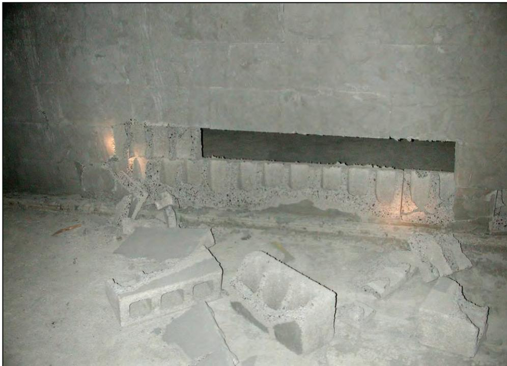
**Figure 46.—Closeup of B-drift side of X-6 dry-stacked hollow-core concrete block stopping after test #430, showing dislodged and damaged blocks. This is clear evidence of roof-to-floor arching action.**
