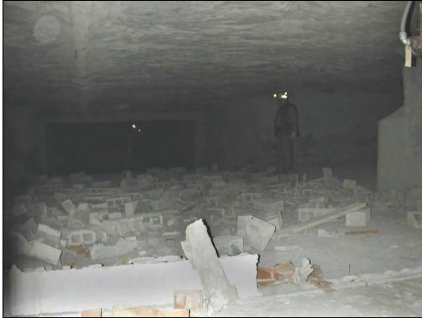
Figure 34.—Debris from dry-stacked hollow-core concrete block stopping in X-4 after LLEM test #428, viewed from C-drift.
