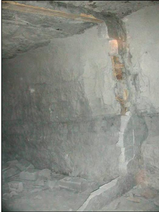
Figure 73.—Debris from the dry-stacked solid-concrete-block stopping and remaining blocks on the inby rib line in X-4 after LLEM test #462, viewed from C-drift.
