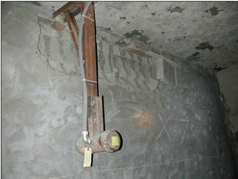
Figure 55.—Expanded view of top part of X-7 dry-stacked hollow-core concrete block stopping after explosion test #433, showing damaged blocks.
