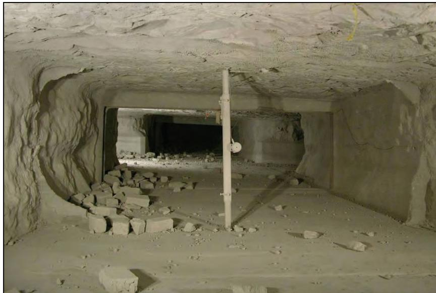
Figure 84.—Debris from 6-in (15-cm) thick, wet-laid solid block stopping in X-7 after LLEM test #519, viewed from A-drift.
