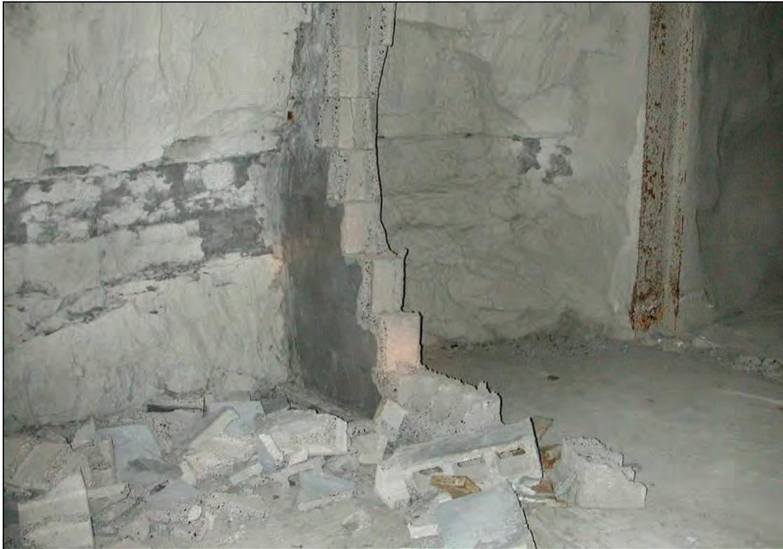
**Figure 39.—Remnants of the dry-stacked hollow-core concrete block stopping in X-5 after LLEM test #428. The block shearing indicates roof-to-floor arching action.**
