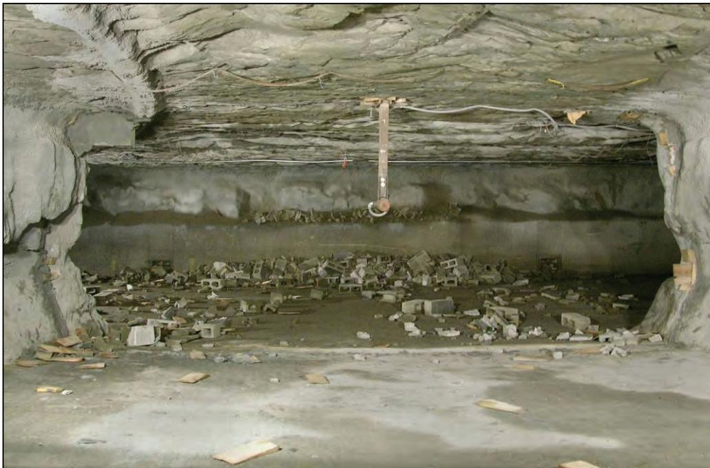
**Figure 92.—Debris from the X-4 dry-stacked hollow-core concrete block stopping between A- and B-drifts after LLEM test #497.**
