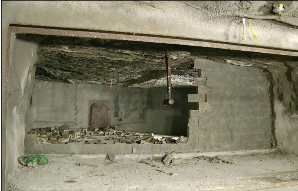
**Figure 91.—Damage to the X-4 dry-stacked hollow-core concrete block stopping between B- and C-drifts after LLEM test #497.**
