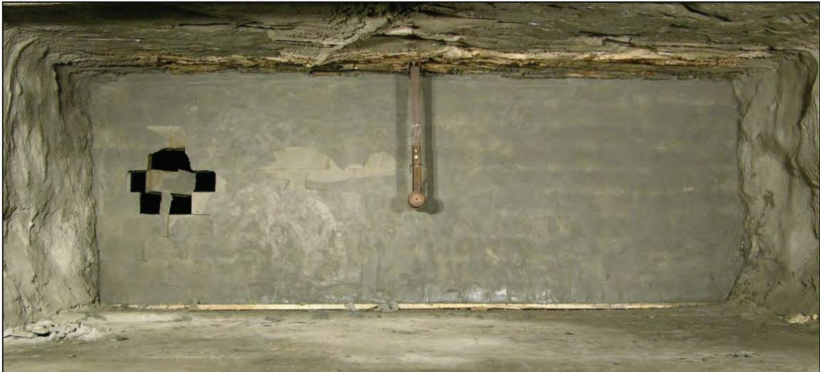
Figure 94.—Damage to the X-3 dry-stacked hollow-core concrete block stopping between B- and C-drifts after LLEM test #497.
