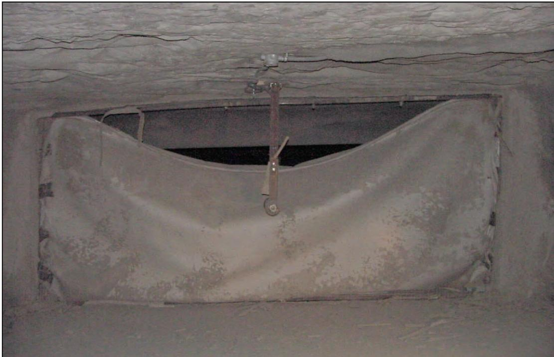
**Figure 106.—Damage to the woven cloth stopping in X-7 after LLEM test #462.**
