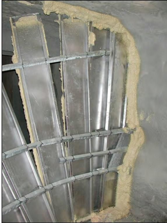
**Figure 67.—Closeup of steel panel stopping still partially attached to outby rib in X-7 after LLEM test #458, viewed from B-drift.**
