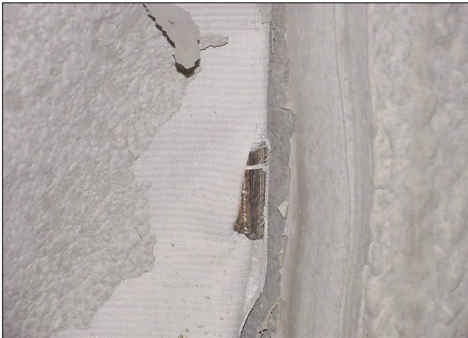
Figure 102.—Initial tear in the woven cloth at the corner steel roof bolt plate position on the inby rib of the X-7 stopping after LLEM test #460, viewed from C-drift.
