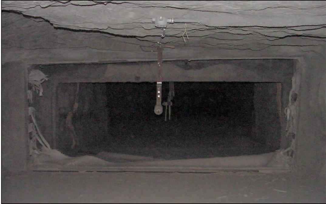
**Figure 105.—Damage to the woven cloth stopping in X-6 after LLEM test #462.**
