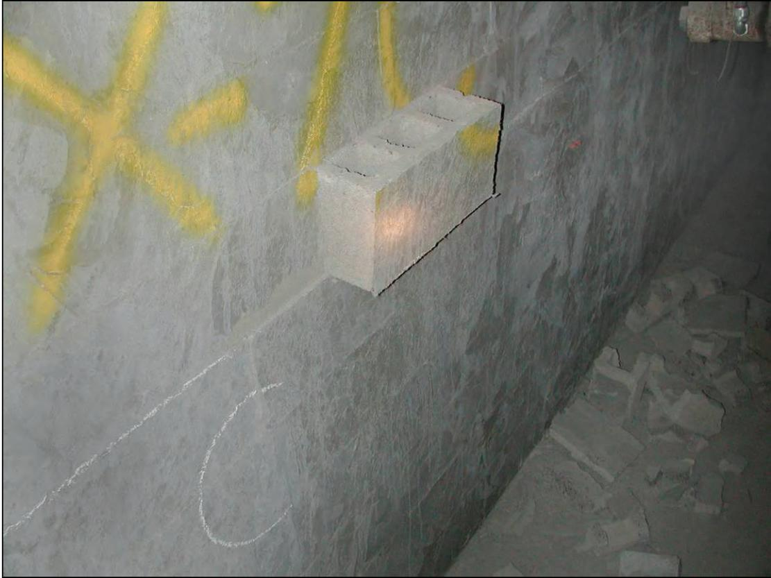
**Figure 56.—Expanded view of hollow-core concrete block that is almost dislodged from X-7 dry-stacked stopping after explosion test #433.**
