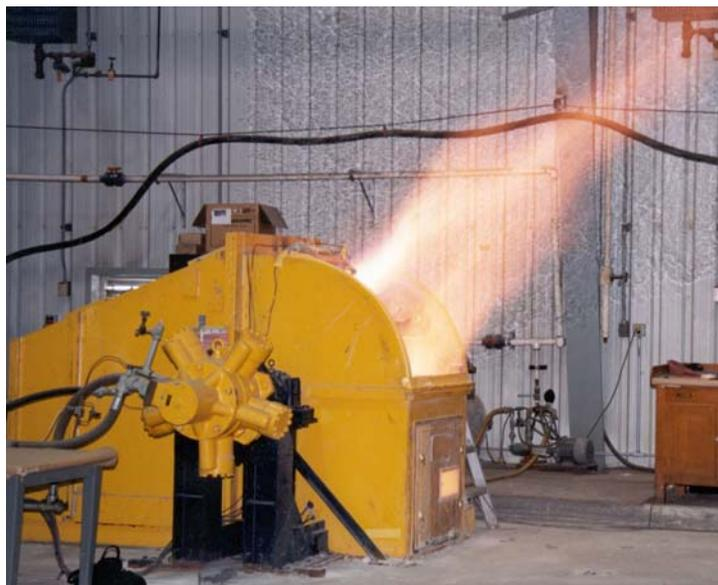
Figure 1.—Frictional ignition of methane in experimental test apparatus.
