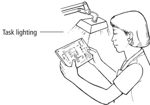
**Provide appropriate lighting** — The quantity and quality of light at your workstation will either serve to enhance or obscure the details of your work. Common problems include:
