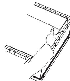
**Provide hand clearance** — Equally important is having sufficient space for the hands in order to avoid "knuckle-buster" injuries and simply to get the job done effectively.
