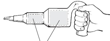
**Dampen vibration and shock** — Working with tools and equipment that create shock or vibration can cause injury. To isolate vibration:
