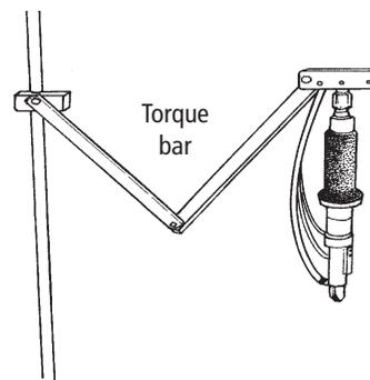
**Use torque bars** — In operations where power screwdrivers and nutrunners are used, it's important to use torque bars and make other modifications to prevent shock from being transferred to the wrists.
