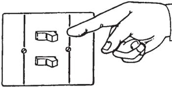
So horizontal switches violate our expectations and provide no hint of correct operation. We don't know automatically which way to flip the switch. By studying issues like this, we can reduce mistakes and confusion.
