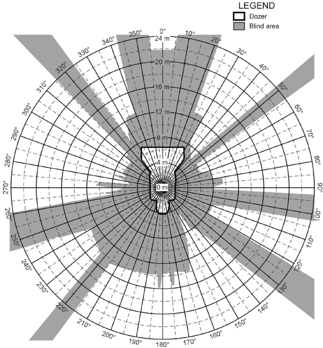
Figure A.11. Blind area diagram for a Caterpillar D11R dozer (ground plane).
