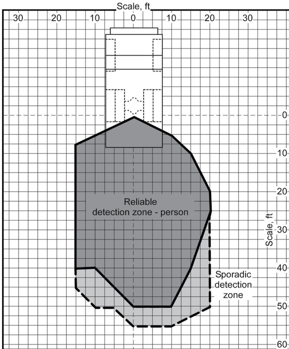
Figure 19. UWB radar detection zone for a person.
