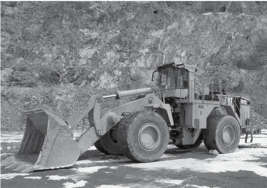
Figure A.4. Caterpillar 992G front-end loader.
