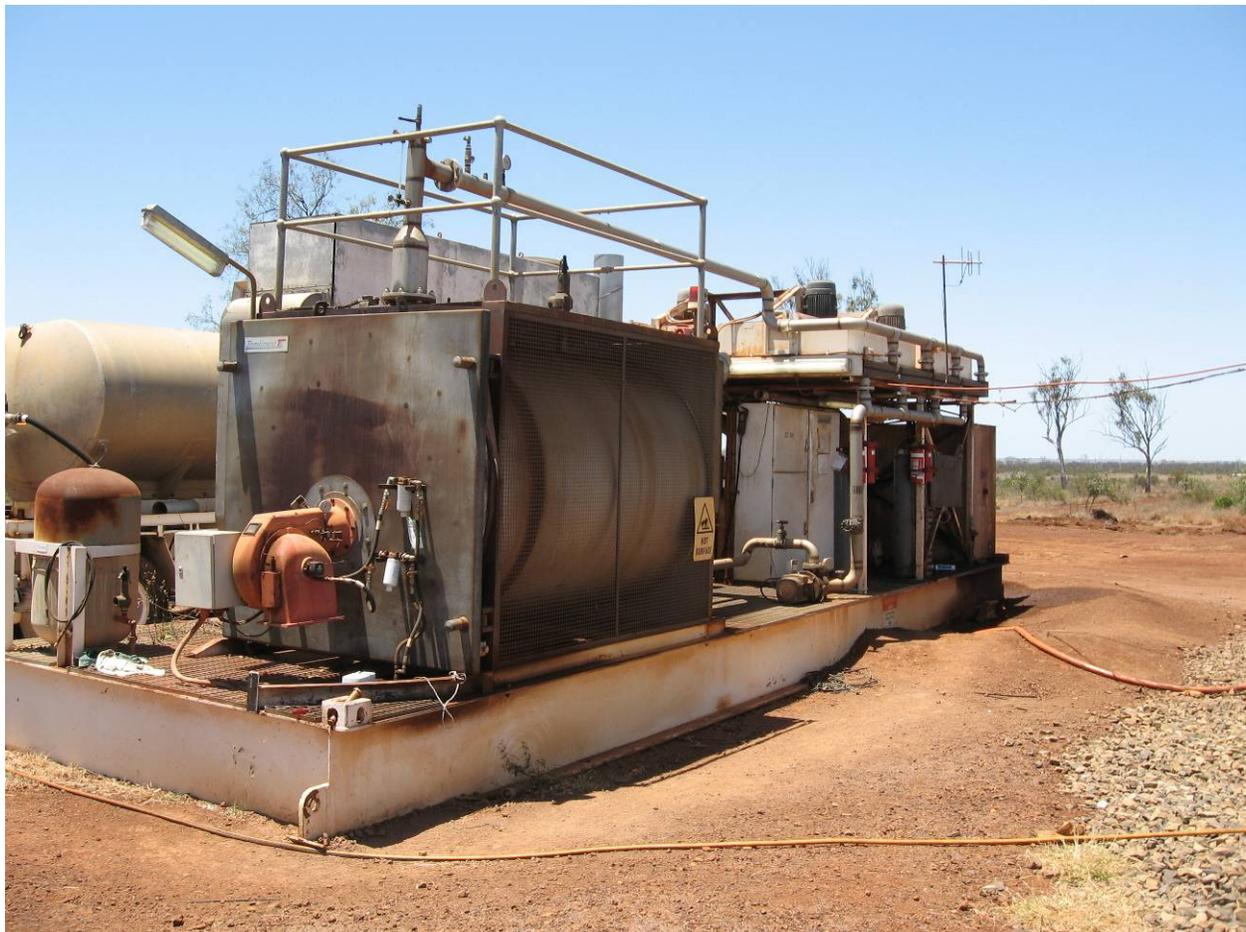
**Figure 9.—Tomlinson boiler for inertization at an Australian coal mine.**
