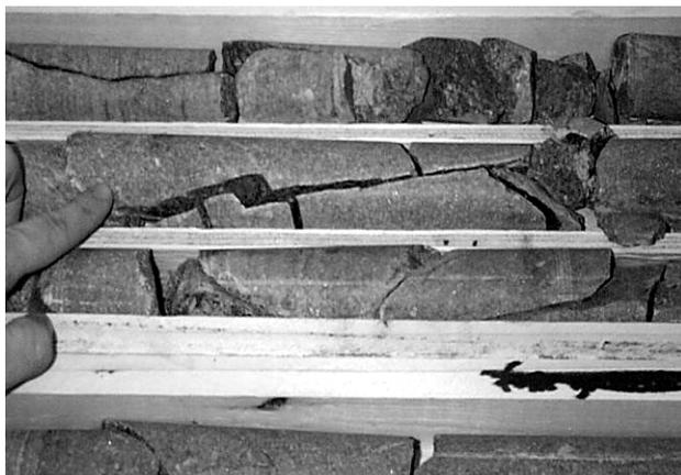
Figure 10.—Joint geometry may not be obvious from the drill core unless the joint is intersected at a very shallow angle.
