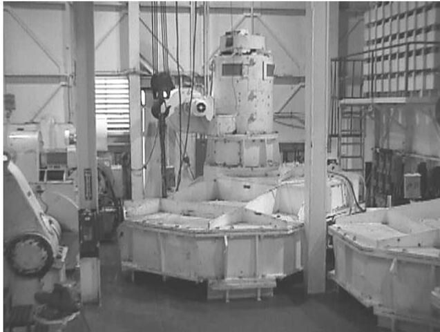
**Figure 17.—Swing motor and gear.**
