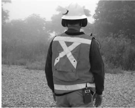
**Figure 4.—Quest Q-400 dosimeter and microphone placement.**
