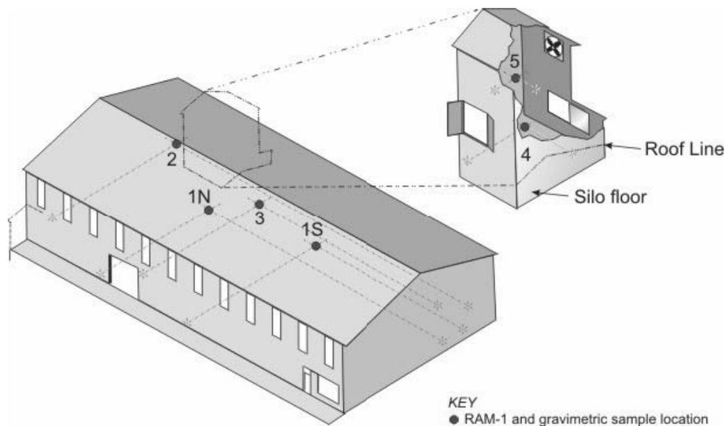
Figure 4.—Dust and noise sampling instrumentation setup at steel-sided structure No. 3.
