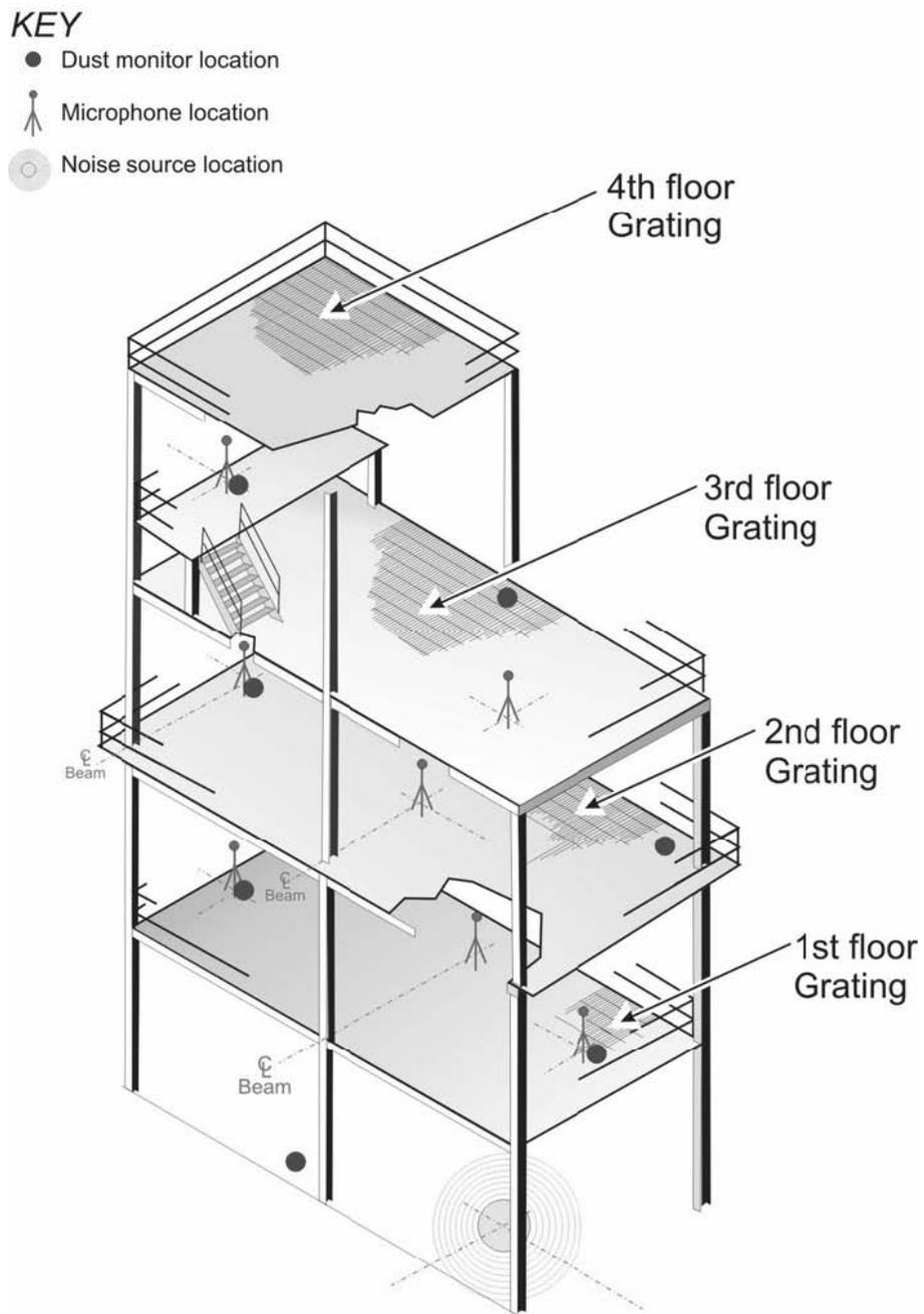
Figure 3.—Dust and noise sampling instrumentation setup at open structure No. 2.
