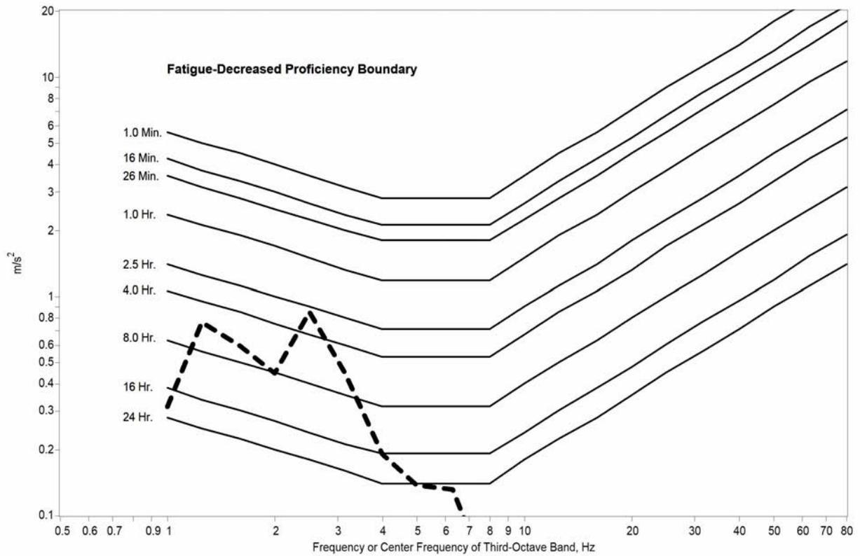
**Figure 16.—Fatigue-decreased proficiency curves for mid-coal-seam shuttle car with NIOSH seat M2B during no-load vehicle operations.**
