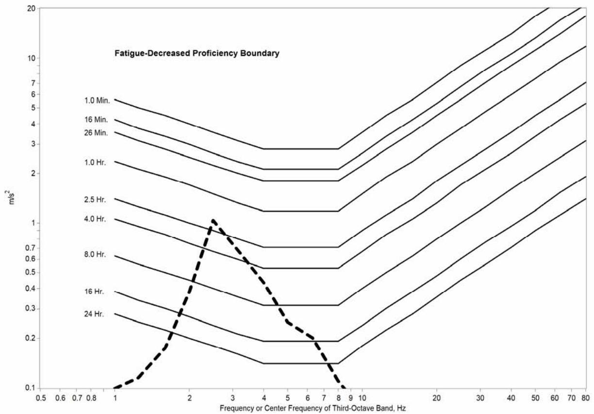
Figure 17.—Fatigue-deceased proficiency curves for low-coal-seam shuttle car with NIOSH seat L2C during no-load vehicle operations.
