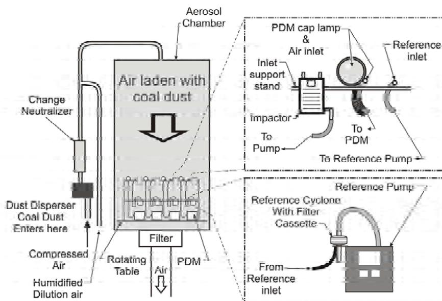
Figure 4.—Laboratory test chamber and arrangement of instruments.
