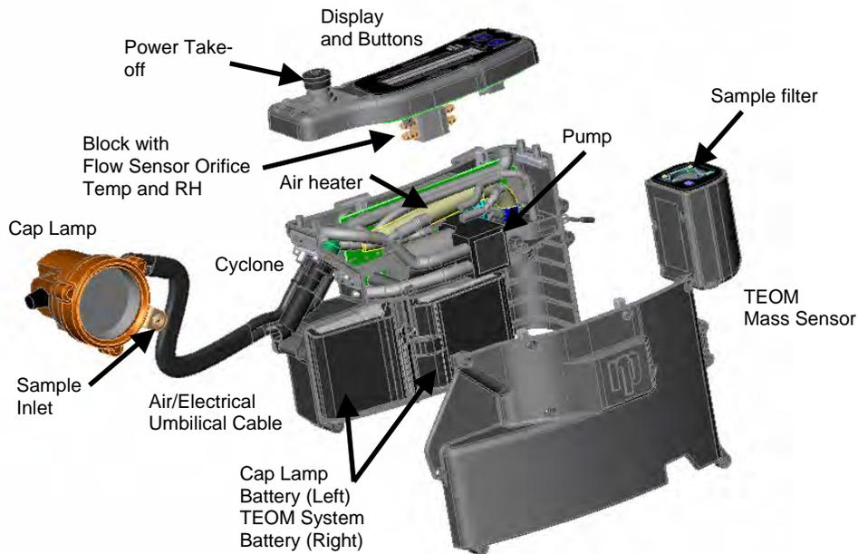
Figure 1.—PDM internal components.
