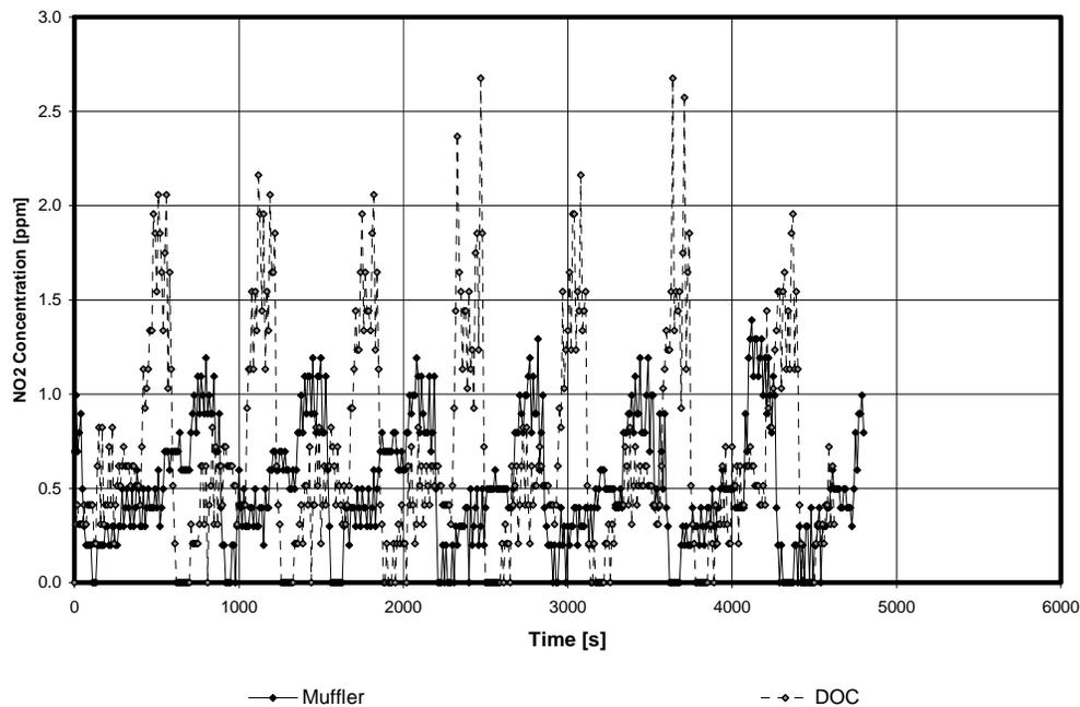
**Figure 20.—Effects of tested DOC on concentrations of NO<sub>2</sub> at vehicle sampling station observed from the test with 50% soy biodiesel (common ventilation rate = 19.28 m<sup>3</sup>/s).**
