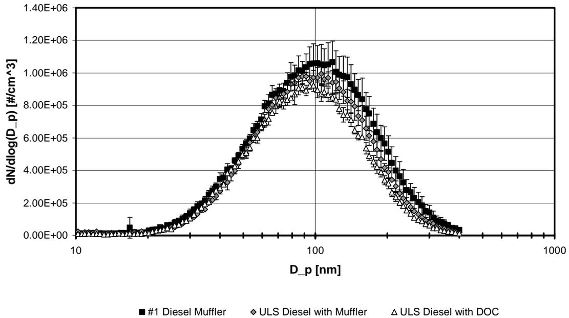
**Figure 19.—Effects of ULS diesel on the size distributions of aerosols (common ventilation rate = 19.28 m<sup>3</sup>/s).**
