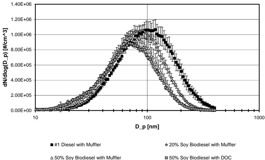
**Figure 17.—Effects of soy biodiesel blends on the size distributions of aerosols (common ventilation rate = 19.28 m<sup>3</sup>/s).**
