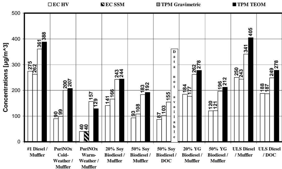
Figure 10.—Contributions of fuel formulation to concentrations of EC and gravimetrically and TEOM-determined TPM (common ventilation rate = 19.28 m<sup>3</sup>/s).
