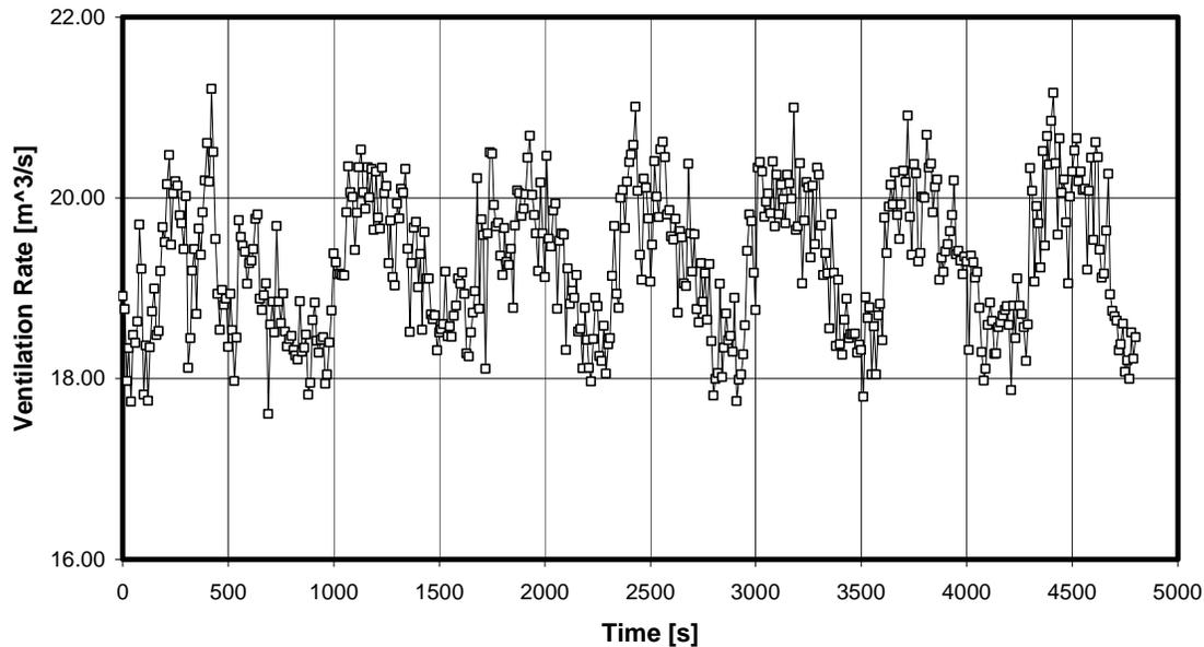
Figure 9.—Ventilation rates measured at the downstream sampling station during the baseline fuel test.
