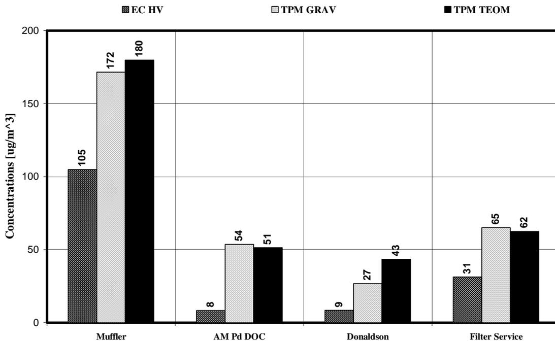
**Figure 22.—VR-adjusted average concentrations of EC and gravimetrically and TEOM-determined TPM (common ventilation rate = 19.29 m<sup>3</sup>/s).**
