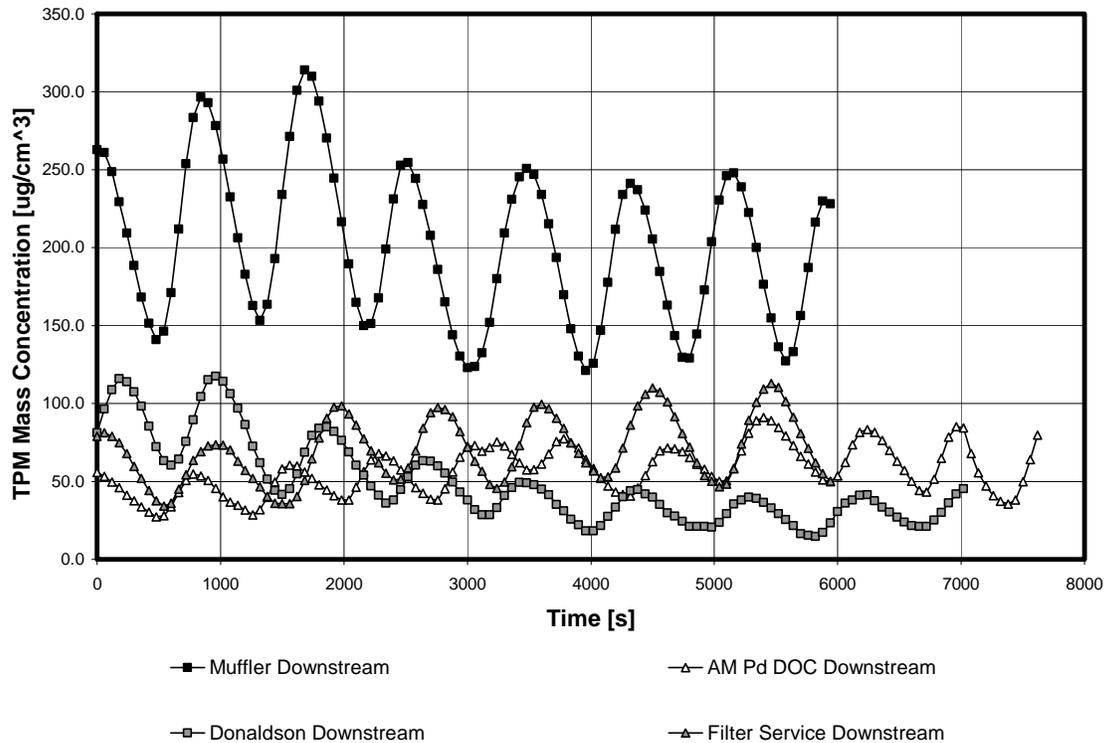
Figure 24.—Effects of filtration systems on mass concentrations of TPM measured throughout the tests by TEOM (common ventilation rate = 19.29 m<sup>3</sup>/s).
