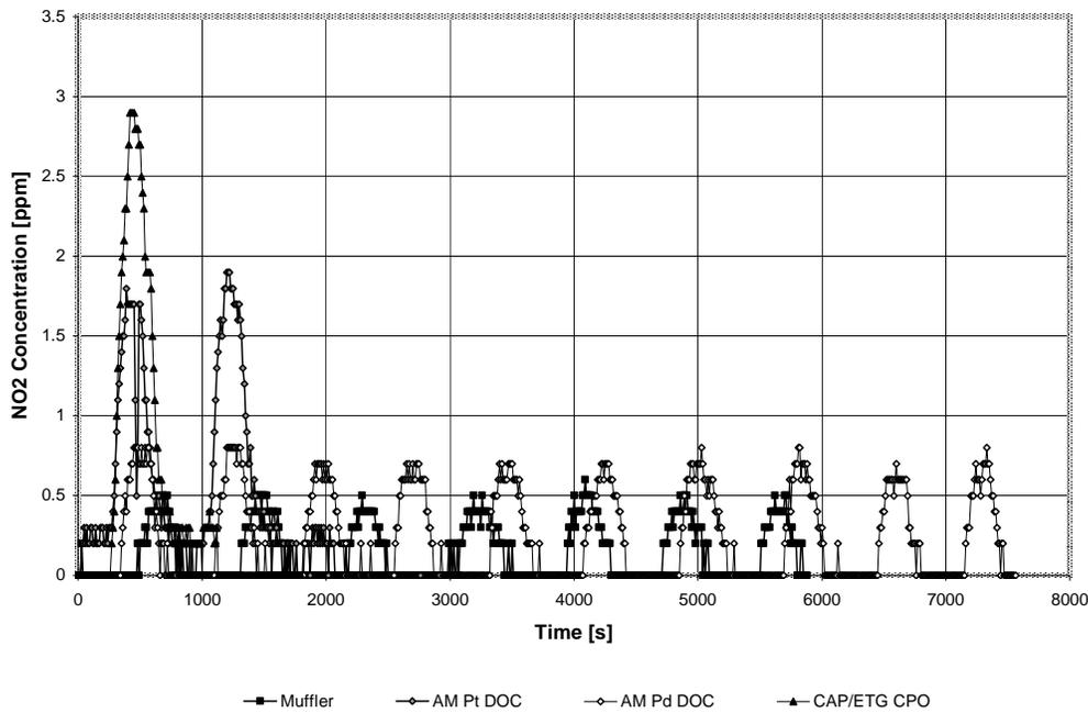
Figure 26.—Effects of filtration systems on NO<sub>2</sub> concentrations at downstream sampling station (common ventilation rate = 19.29 m<sup>3</sup>/s).
