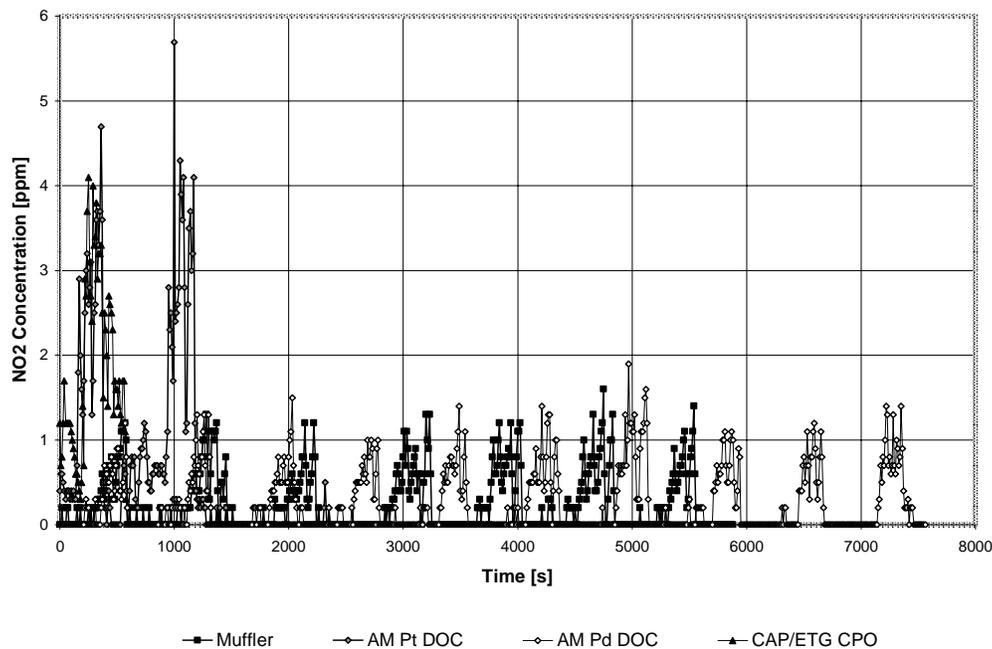
**Figure 27.—Effects of filtration systems on NO<sub>2</sub> concentrations at vehicle sampling station (common ventilation rate = 19.29 m<sup>3</sup>/s).**
