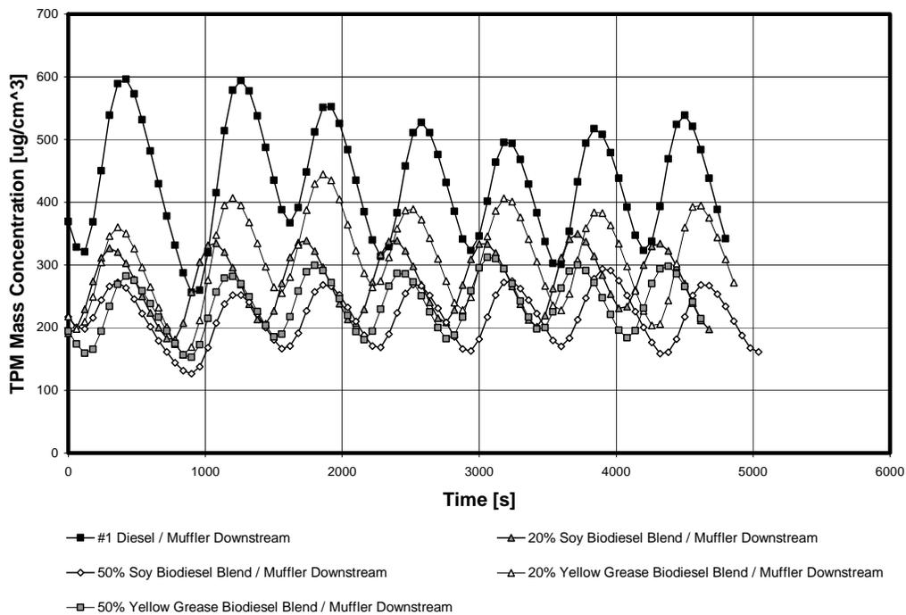
**Figure 13.—Effects of biodiesel blends on mass concentrations of TPM at downstream sampling station measured by TEOM.**
