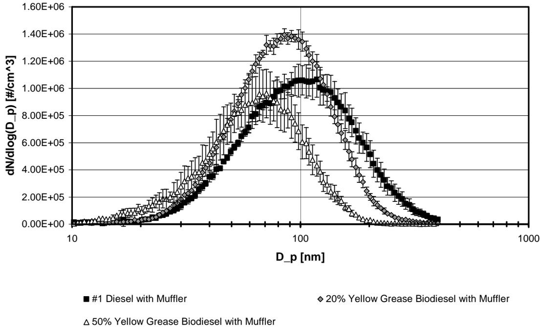
**Figure 18.—Effects of yellow grease biodiesel blends on the size distributions of aerosols (common ventilation rate = 19.28 m<sup>3</sup>/s).**
