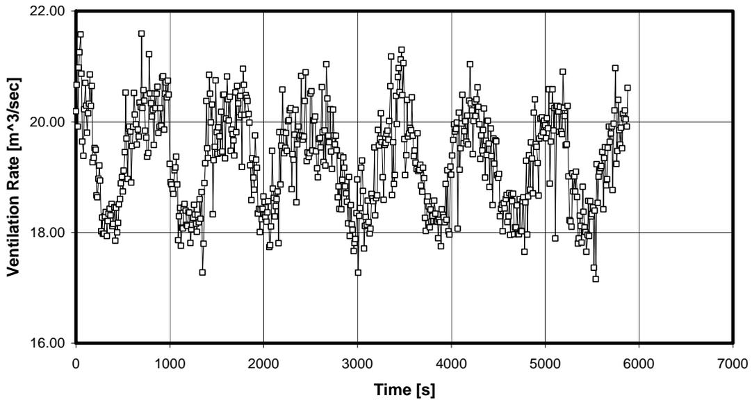
Figure 21.—Ventilation rates measured at the downstream sampling station during the baseline filter test.
