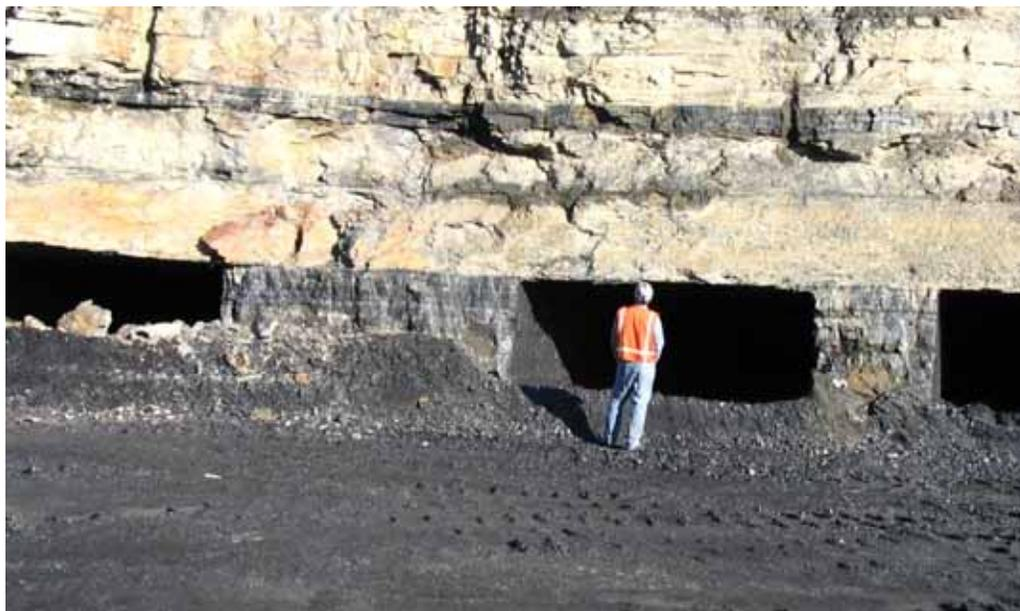
Figure 1.—Highwall mining, showing a barrier pillar (left) and a web pillar (right).
