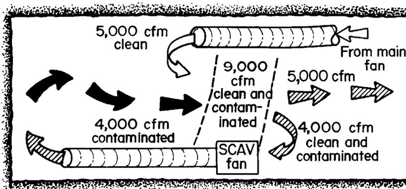
Figure 14–8.—Loss of efficiency from mismatched airflow directions.
