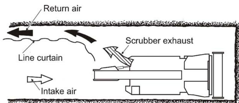
58 cfm, depending on airflow.<sup>12</sup> Both of these studies employed an exhaust line curtain located on the *same* side of the entry, so the air jet from the scrubber fed directly into the line curtain as shown in Figure 3-10.
