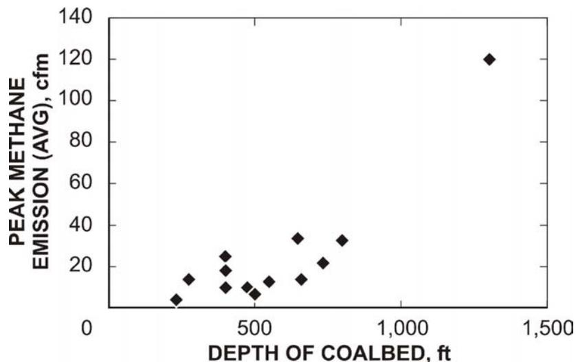
peaks, not the overall methane level. Figure 3-2 shows peak average<sup>4</sup> methane emissions in several U.S. coalbeds [Haney et al. 1983]. Except for one coalbed at 1,300 ft depth, peak average coalbed emissions range from 4 to 33 cfm, with an overall U.S. average of 17 cfm. Any face ventilation system must be able to safely handle gas flows of this magnitude.
