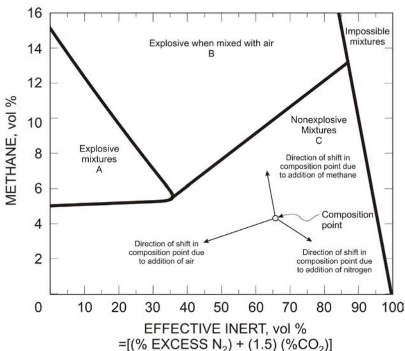
Figure 1-2.—Methane explosibility diagram (from Zabetakis et al. [1959]).
