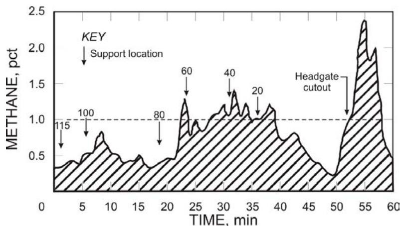
Figure 4-3.—Methane concentration at shearer during tail-to-head pass.
