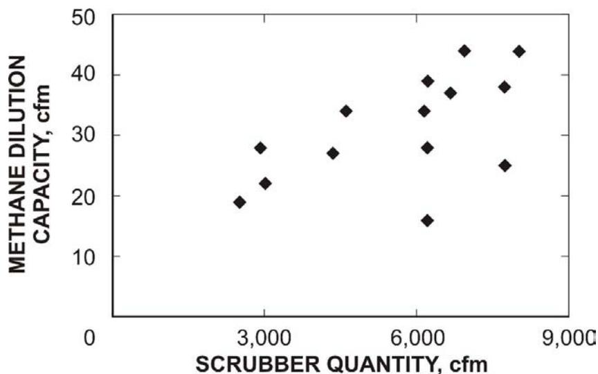
Figure 3-8.—Methane dilution capacity from MSHA scrubber tests.
