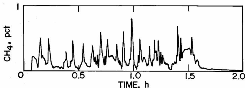
These methane peaks can be substantial. For this reason, efforts to safely dilute the methane must focus on the level of the
