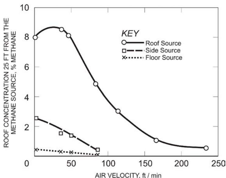
**The rib and floor as sources of methane layers.** Methane layering occurs when methane is released at the mine roof. When methane is released at the mine floor or rib, this gas readily mixes into the ventilation air stream, losing its buoyancy. Figure 1-6, from Bakke and Leach [1962], compares 2-cfm methane sources at the roof, rib, and floor of the mine entry. Only the roof source produced a significant methane layer at the 2-cfm rate.<sup>26</sup>
