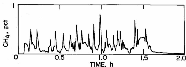
Figure 2-3.—Recorder chart from a machine-mounted methane monitor.
