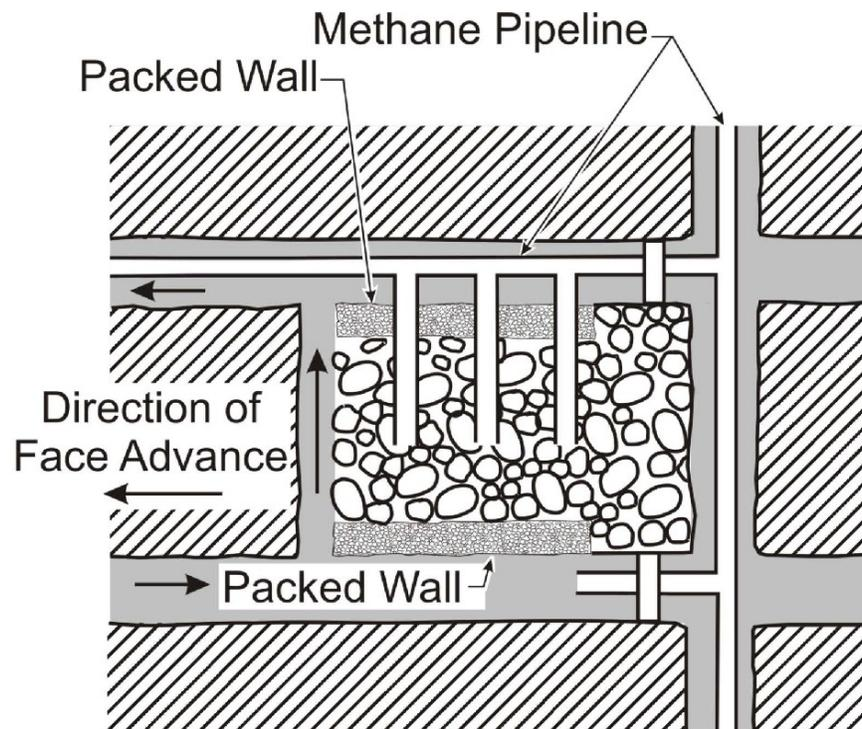
Figure 6-7.—Methane drainage by the packed cavity method.
