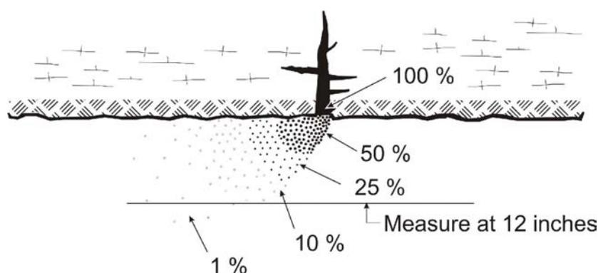
hazard exists. This problem is handled by requiring methane measurements at a distance of not less than 12 in from the roof, face, ribs, and floor. If there is enough gas coming from the crack (or other source) to exceed statutory limits at a 12-in distance, then a hazardous condition exists.
