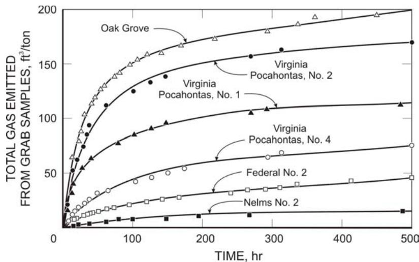
Figure 11-2.—Gas emitted from conveyor belt grab samples.
