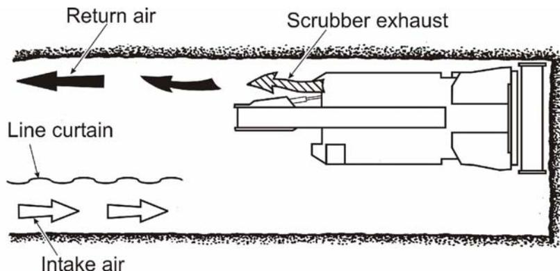
Figure 3-7.—Dust scrubber used in conjunction with blowing ventilation.
