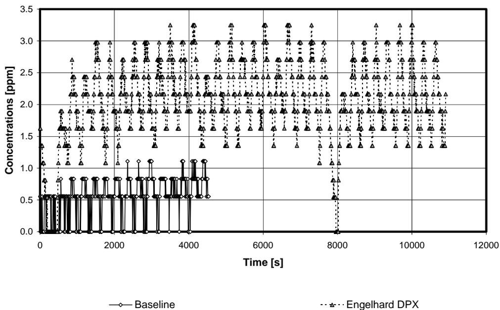
Figure 32.—Normalized NO<sub>2</sub> concentrations at the downstream sampling station for the tests with haul truck #92128.
