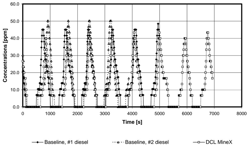
Figure 31.—Normalized NO concentrations for the tests with LHD #99942.
