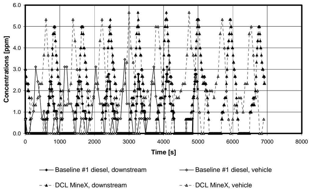
**Figure 34.—Normalized NO<sub>2</sub> concentrations at the downstream and vehicle sampling stations for the baseline (#1 diesel) and DCL MINE-X DPF system tests with LHD #99942.**
