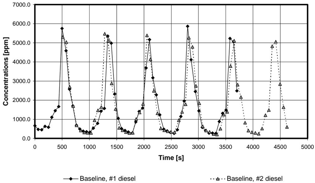
Figure 27.—Normalized CO<sub>2</sub> concentrations for the tests with LHD #92506.
