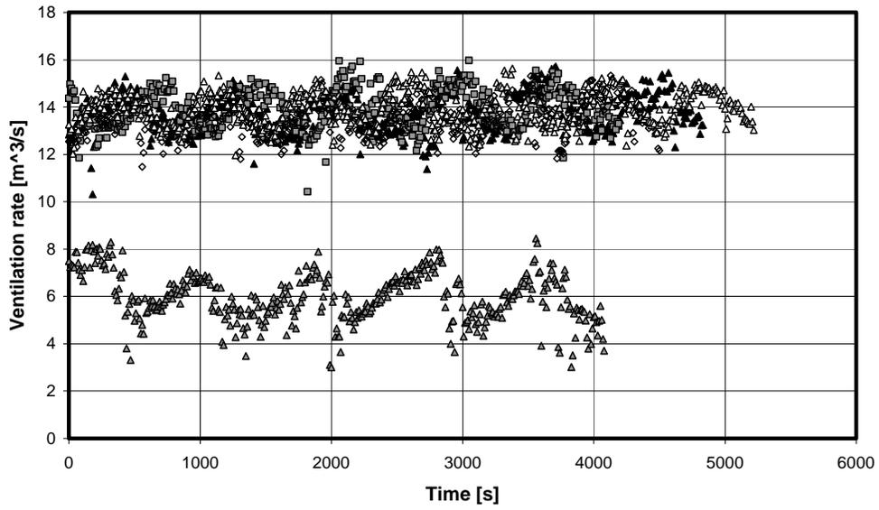
Figure 18.—Ventilation rates for the tests involving #92526.
