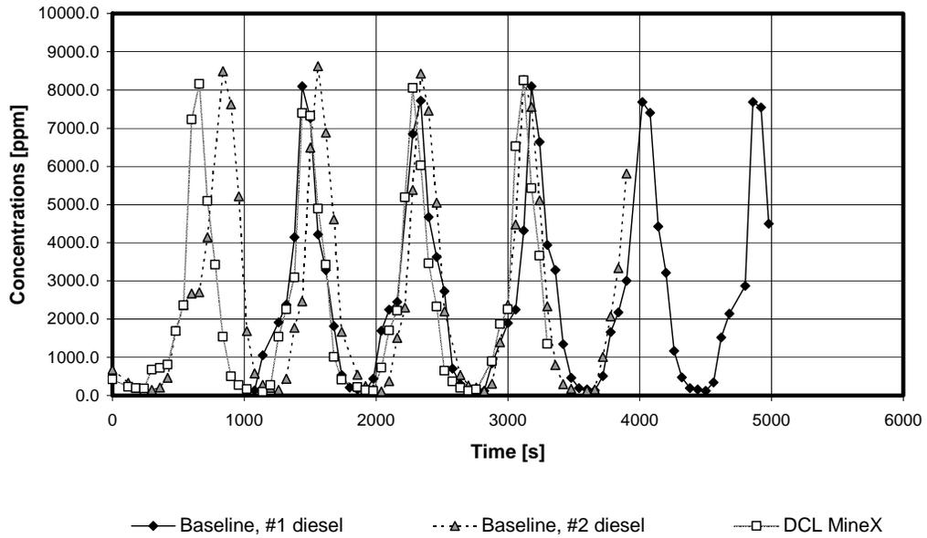
Figure 29.—Normalized CO<sub>2</sub> concentrations for the tests with LHD #99942.
