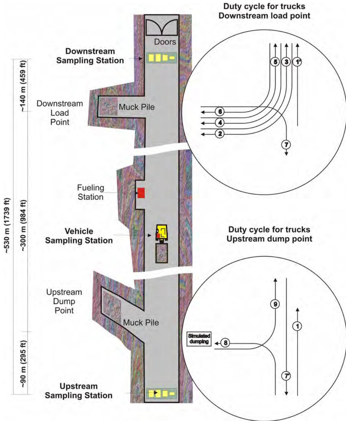
Figure 10.—The isolated zone and duty cycles for trucks #92128 and #92133 (not to scale).
