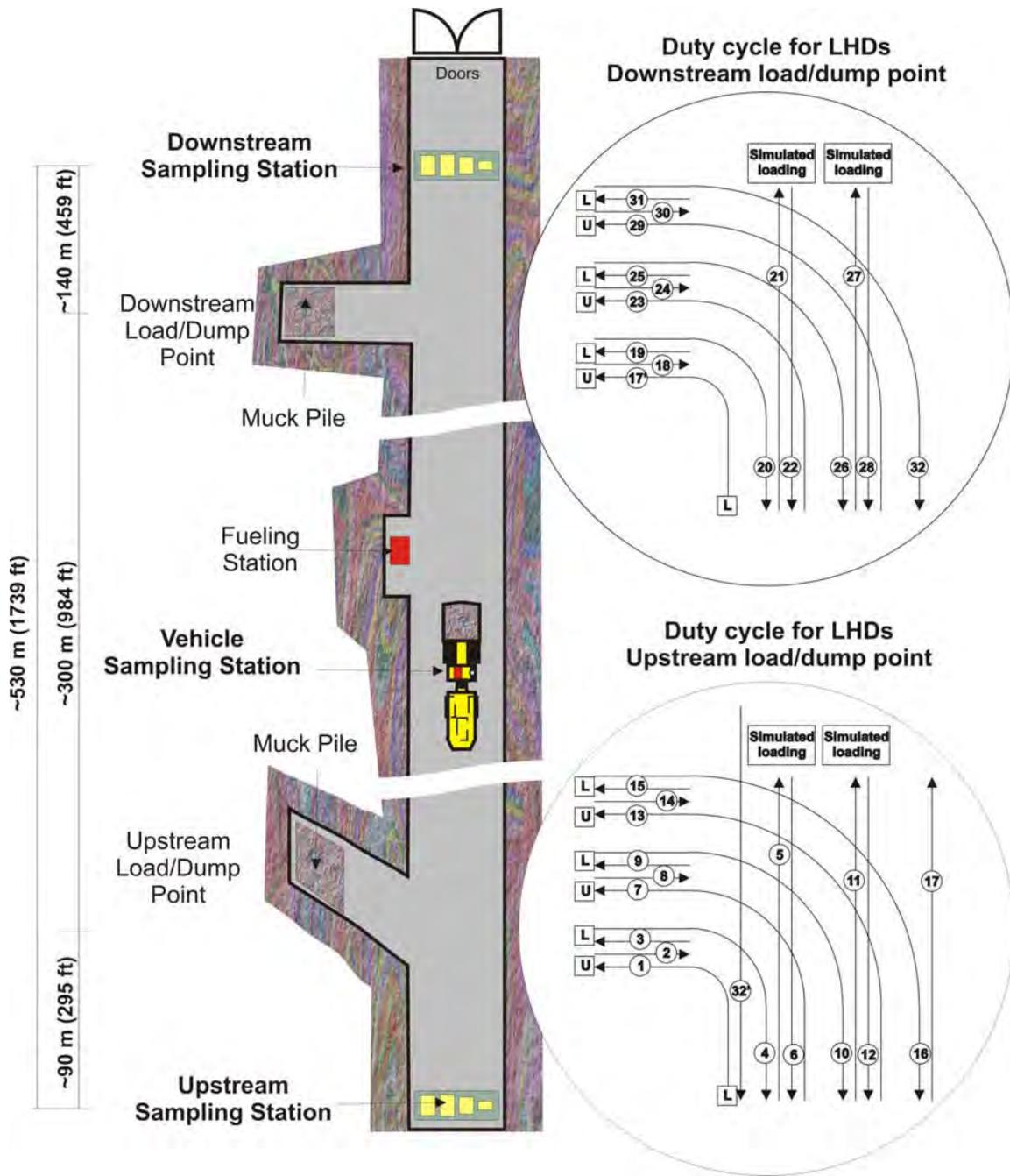
Figure 11.—The isolated zone and duty cycles for LHDs #92506, #92526, and #99942 (not to scale).
