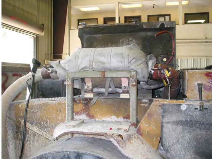
Figure 2.—CleanAIR Systems DPF system on truck #92133.
