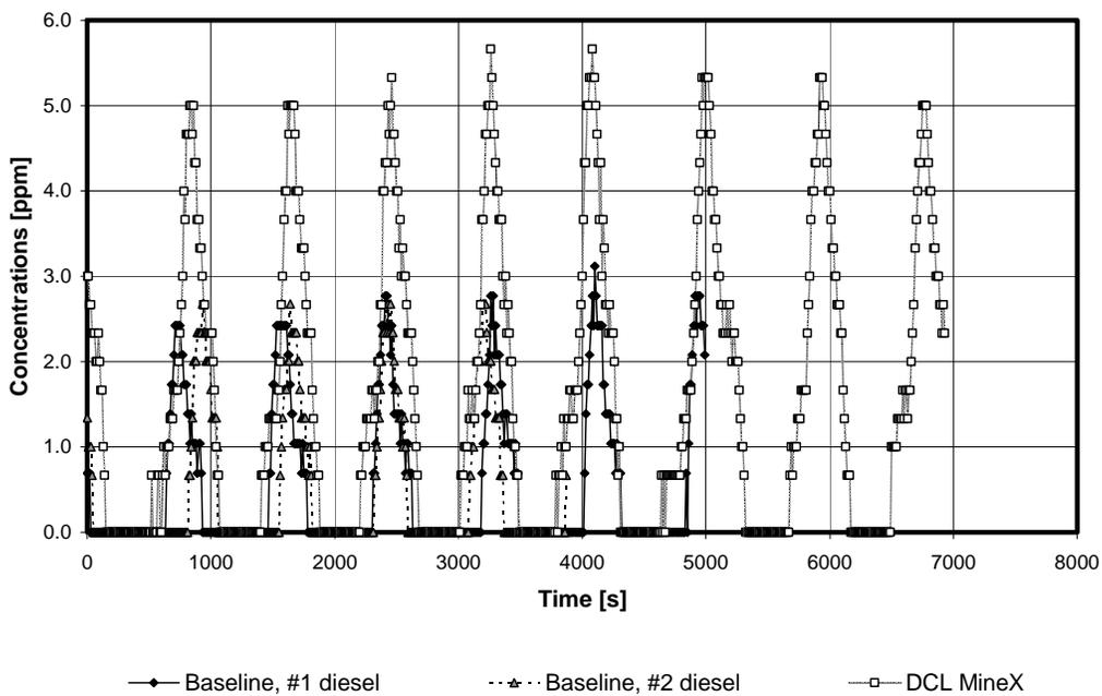
Figure 33.—Normalized NO<sub>2</sub> concentrations at the downstream sampling station for the tests with LHD #99942.
