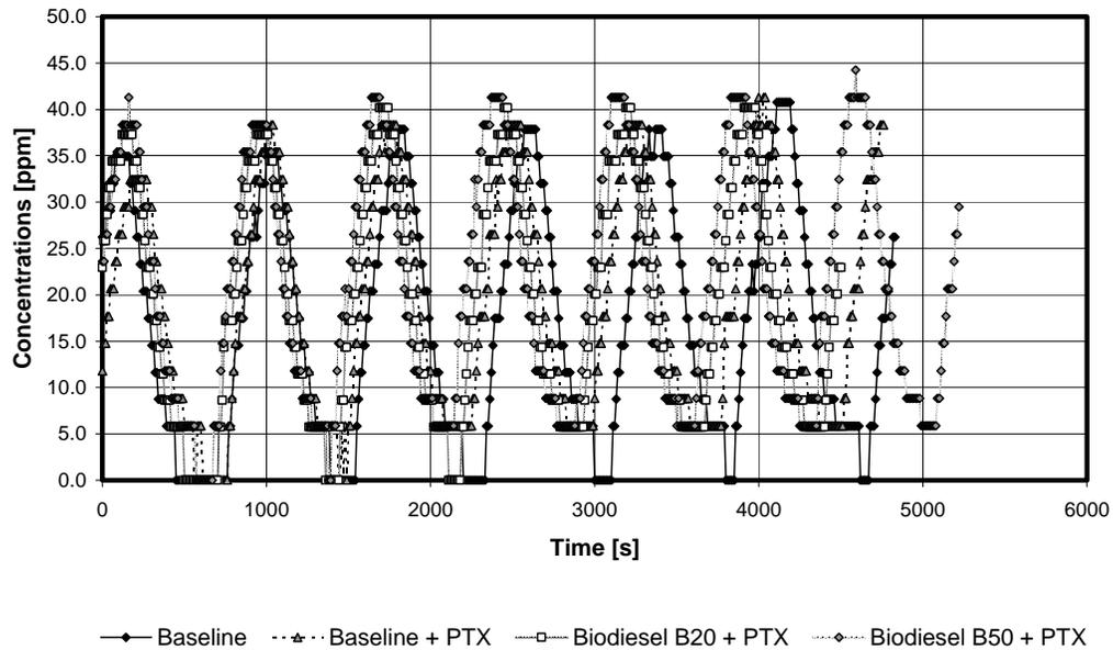
Figure 30.—Normalized NO concentrations for the tests with LHD #92526.
