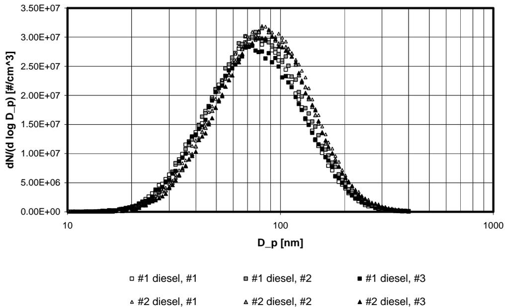
**Figure 26.—Size distribution of aerosols in mine air for LHD #99942 equipped with muffler: #1 diesel and #2 diesel (three measurements each).**
