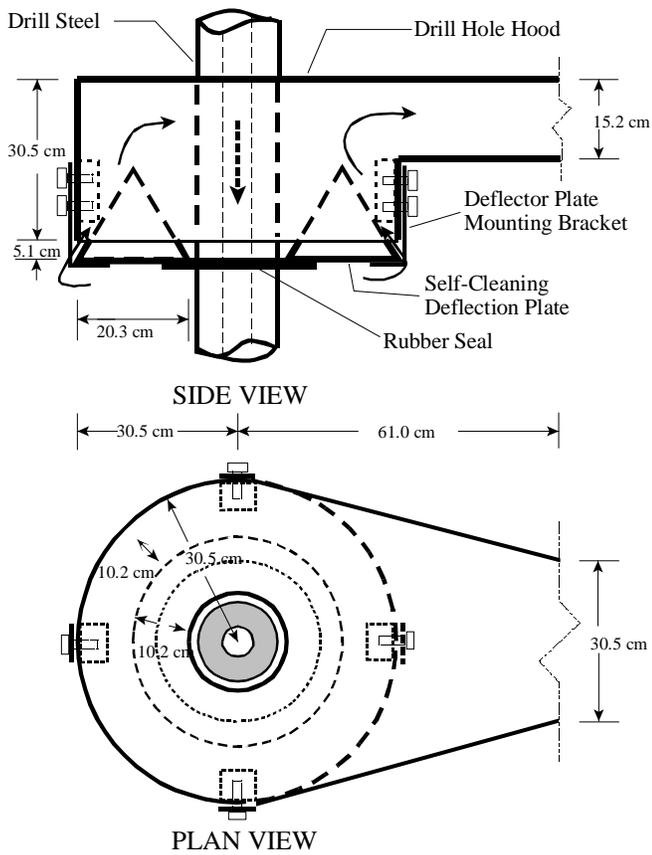
Figure 1. Inlet hood design tested in laboratory.
