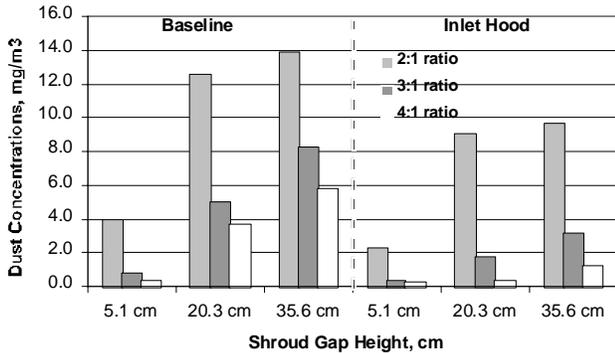
Figure 2. Dust escaping the laboratory drill shroud.
