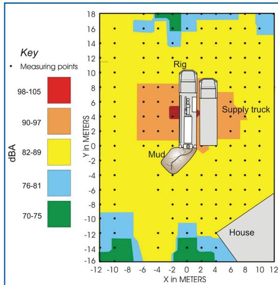
**Figure 1.** The image above shows sound levels around a typical water well worksite. In this example, workers are exposed to sound levels above 90dB(A) within 6 meters of the rig, particularly near the compressor. All workers at a worksite should always wear hearing protection and avoid standing in these areas if not required to conduct a work task.
