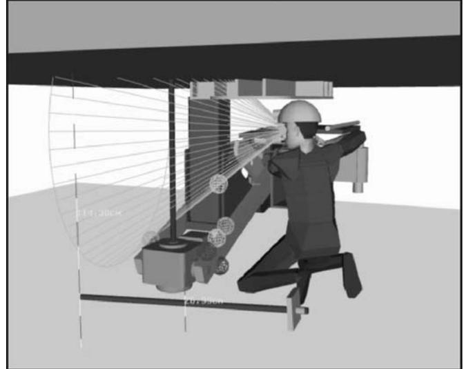
Figure 9.–Virtual operator's behavior hand off drill and boom arm.
