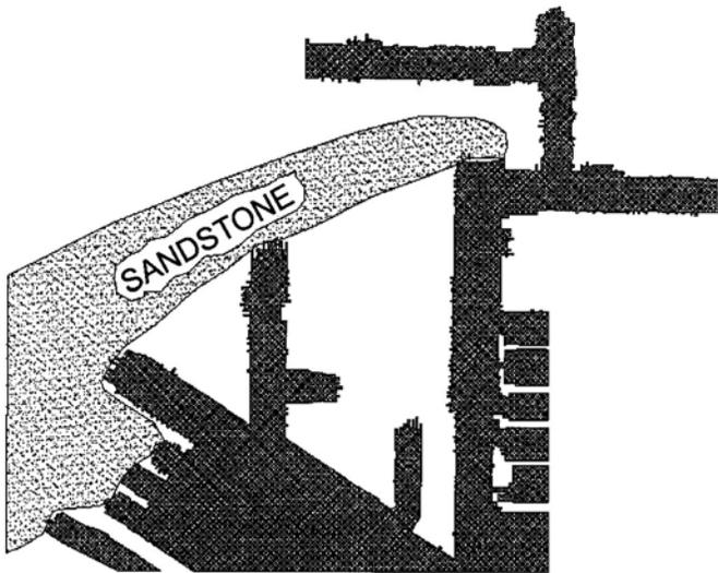
Figure 33.—Complete washout of the coal by a paleochannel in a West Virginia mine terminated numerous headings.
