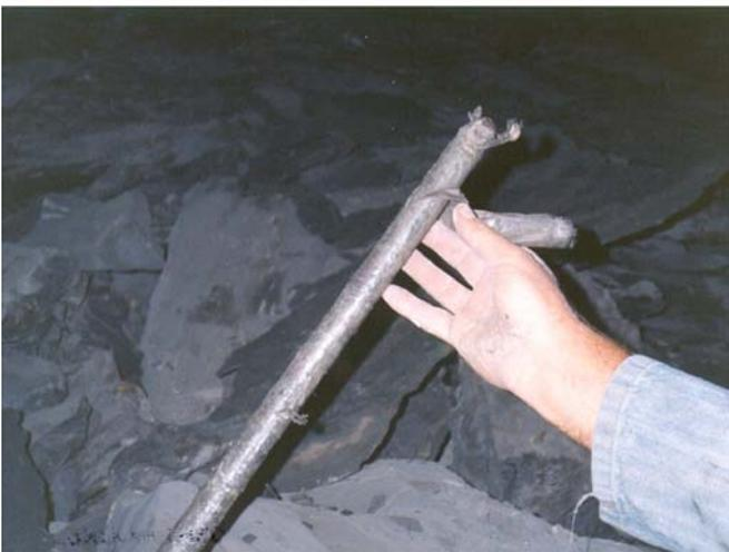
Figure 46.—Two views of "glove-fingered" bolts that provide little mechanical interlock to support strata.
