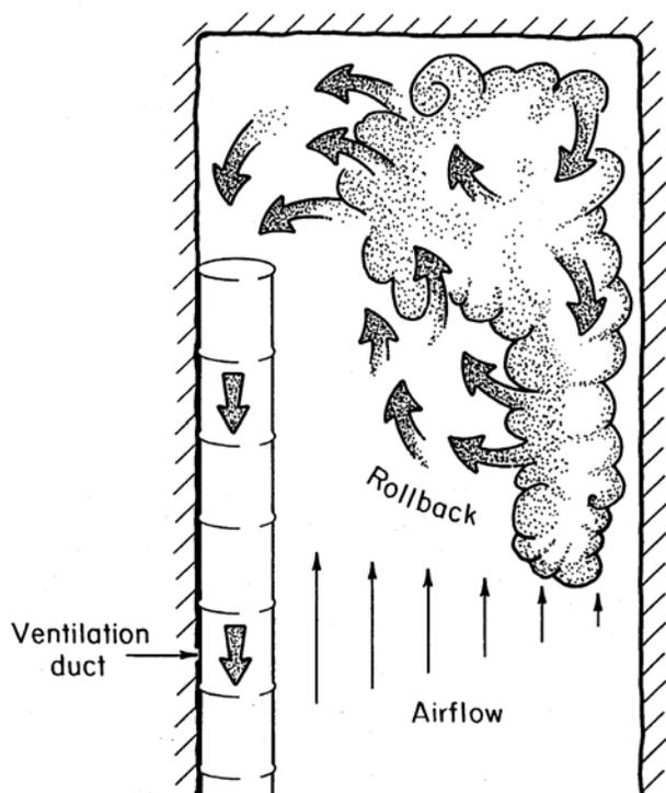
Figure 1-1.—Rollback of dust resulting from non-uniform airflow.
