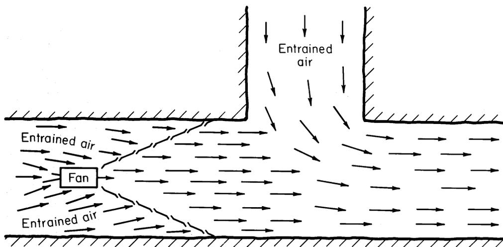
Figure 4-3.—Jet fan entrainment of mine air.
