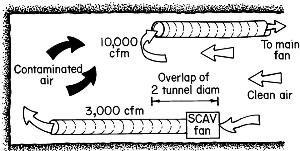
Figure 7-3.—Auxiliary, or scavenger, system with adequate overlap.
