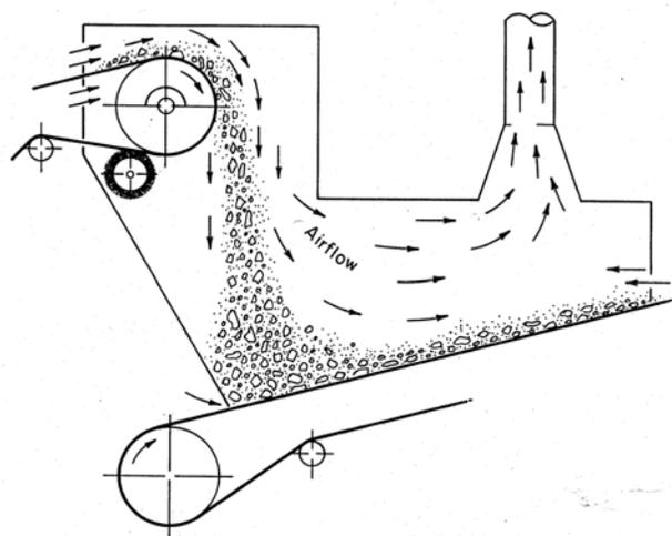
**Figure 6-4.—Dust-laden air exhausted from transfer point enclosure.**
