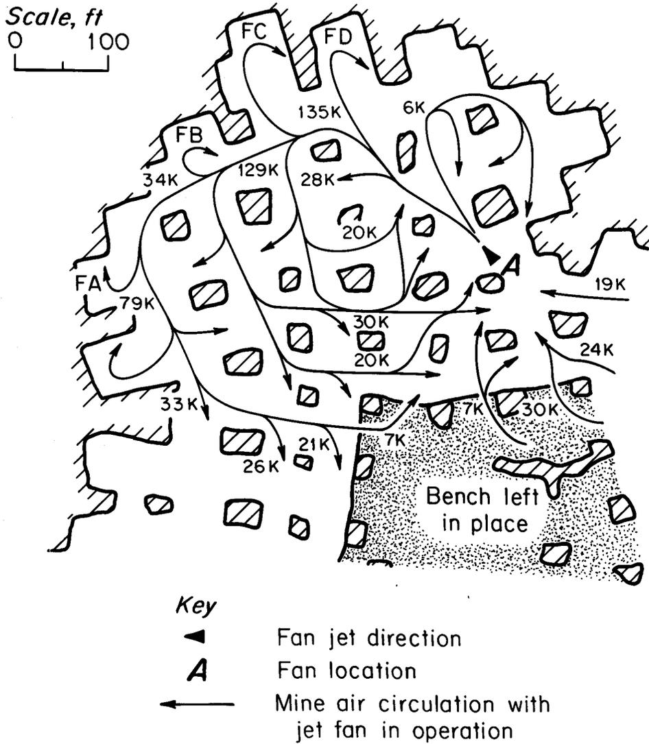
Figure 4-5.—Airflows obtained with jet fan in operation.
