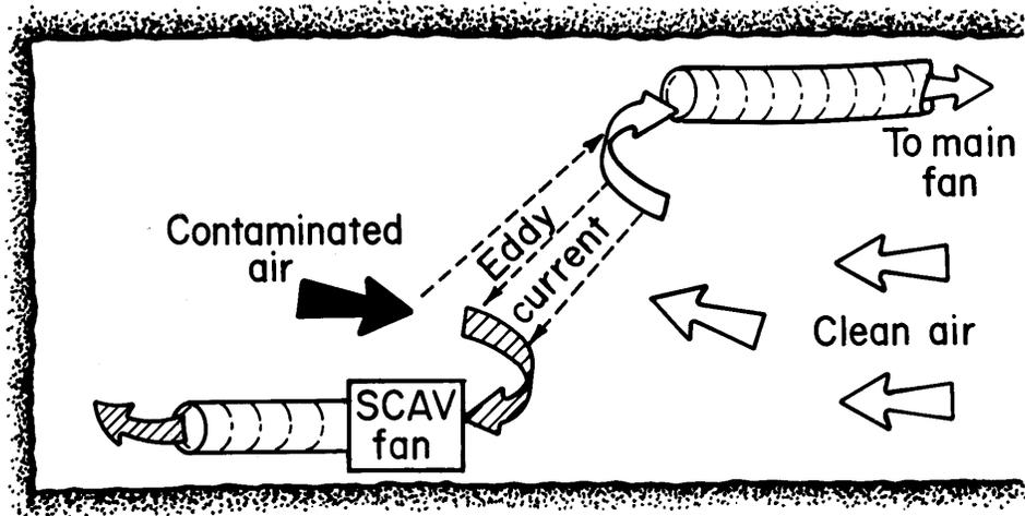
Figure 7-4.—Auxiliary, or scavenger, system with no overlap.
