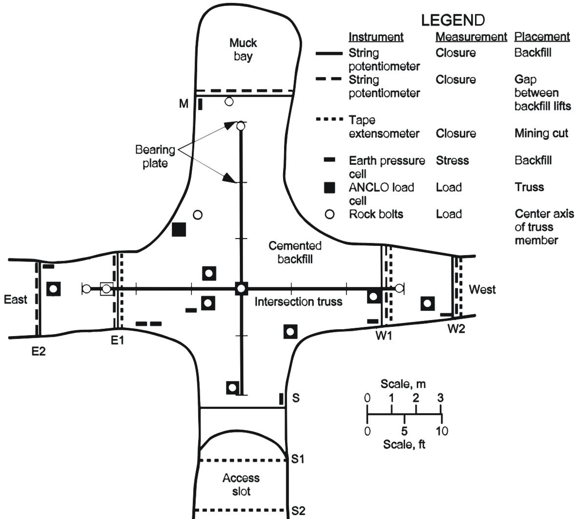
Figure 5.—Location of instruments in 5660-05-level intersection.
