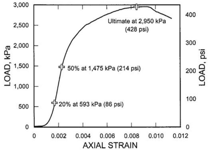
Figure 11.—Compressive test of cemented sandfill, stress/strain curve.
