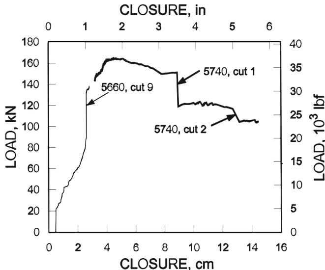
Figure 14.—Backfill closure versus rock bolt load, East 2.
