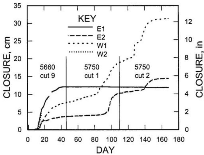
Figure 10.—Backfill closure as a function of time.
