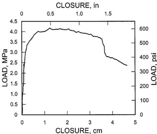
Figure 12.—Backfill closure versus backfill pressure, West 2.
