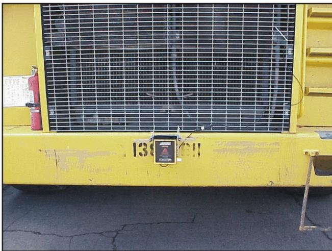
Figure 11.—Ogden radar system mounted on front bumper.
