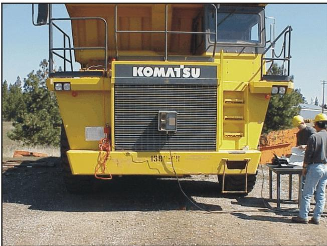
Figure 29.—Ultrawide-band radar system mounted on front grill.
