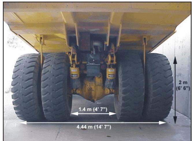
**Figure 2.—Rear view of Komatsu 210M.**
