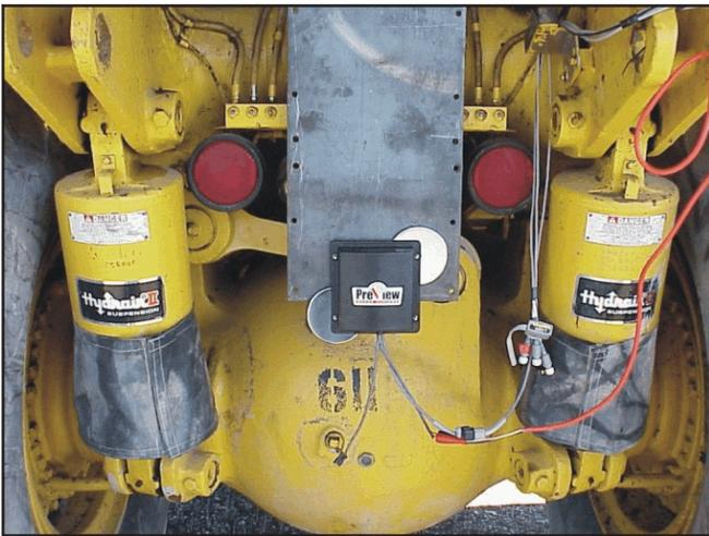
**Figure 18.—Preview radar system antenna and electronics enclosure.**
