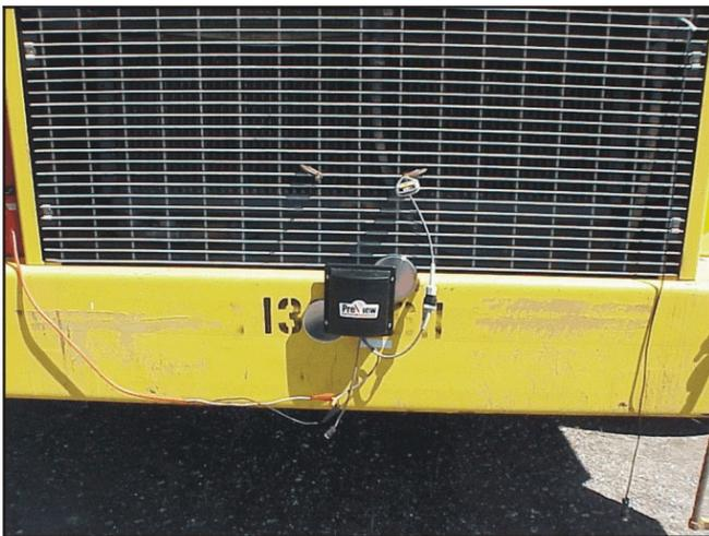
Figure 22.—Preview radar system mounted on front bumper.
