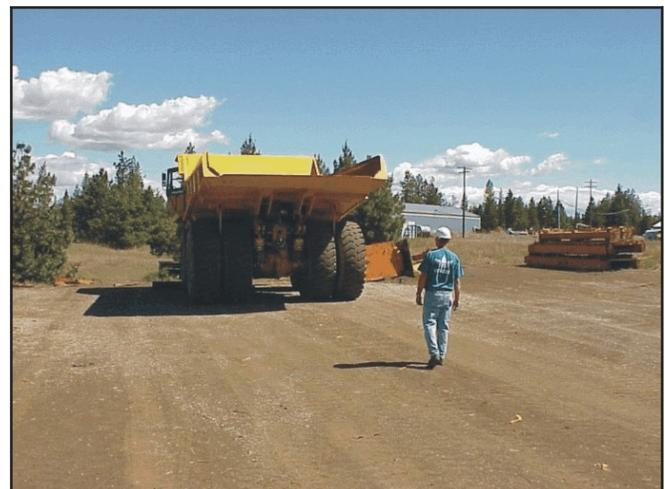
**Figure 3.—Determining detection zone for a person.**
