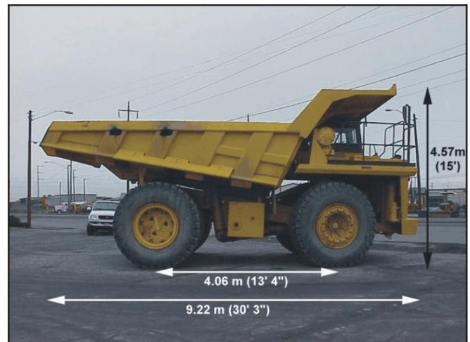
Figure 1.—Side view of Komatsu 210M.
