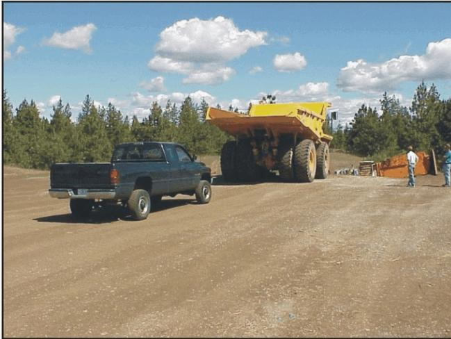
Figure 4.—Determining detection zone for a pickup truck.
