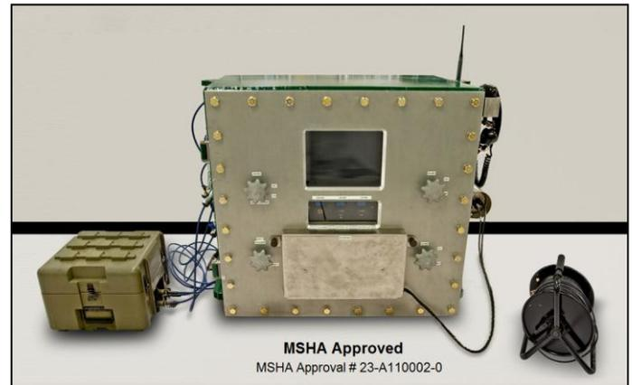
Figure 2. MagneLink® Magnetic Communications System.
