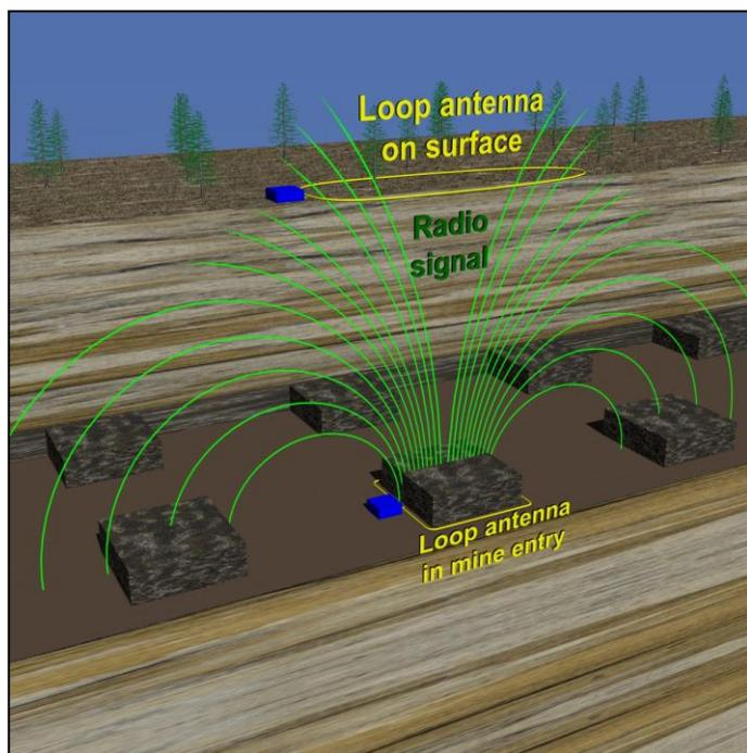
Figure 1. An example of through-the-earth (TTE) communications depicted at a mine site.
