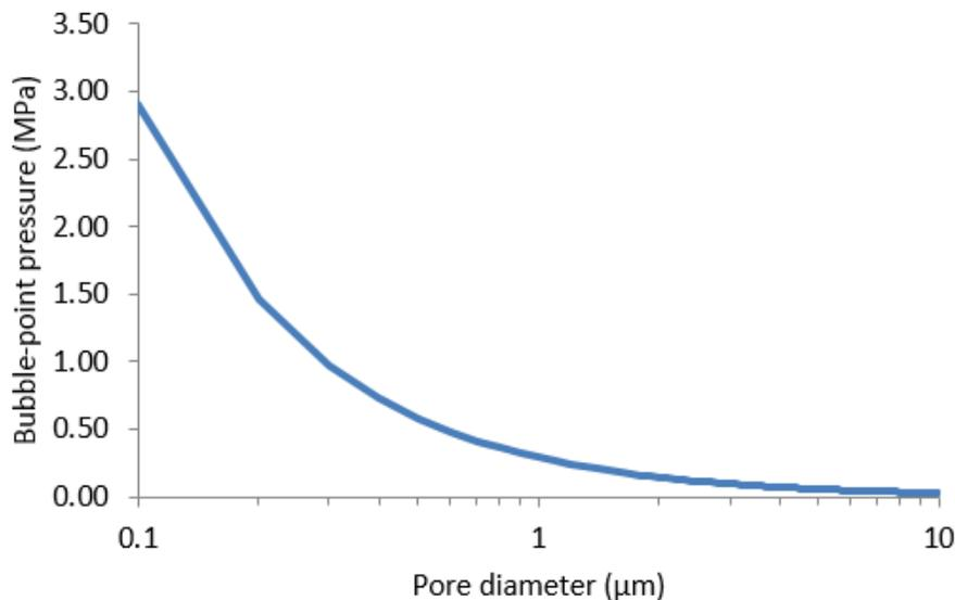
**Figure 3: Pore diameter vs. air pressure for ideal filter in bubble-point test. The curve was calculated with use of water (which has a surface tension of 72.8 mN/m) as the liquid. It is assumed that the water completely wets the filter material, and thus the contact angle  $\theta = 0^\circ$ . Calculated using Equation 1.**
