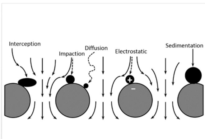
**Figure 4: Aerosol particle collection mechanisms. Different types of filters have different structures but they all collect particles using the mechanisms shown here. The relative importance of the various collection mechanisms depends upon the size, shape, density and electrostatic charge of the aerosol particles and the velocity of the air flow through the filter.**
