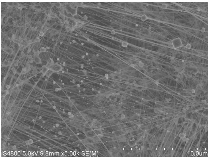
**Figure 7: NaCl aerosol particles collected using a PTFE porous membrane filter with a 3- $\mu\text{m}$  equivalent pore diameter at a face velocity of 8.3 cm/s. As can be seen, particles much smaller than 3  $\mu\text{m}$  were captured by the filter.**
