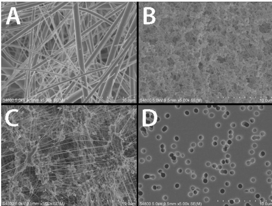
**Figure 1: Scanning Electron Micrographs (SEM) of four filter types. The vertical tick marks above “10.0 µm” in the lower right-hand corner of each SEM are 1 µm apart; the entire scale is 10 µm in length.**
