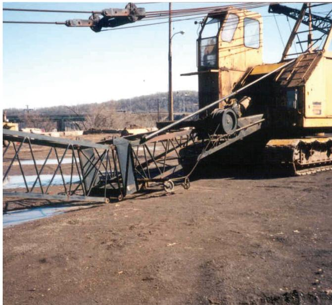
Boom collapse during crane disassembly.
