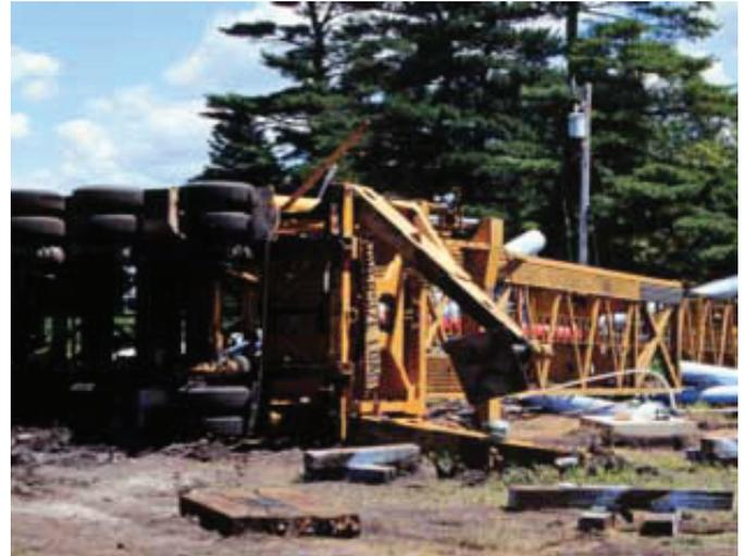
Mobile tower crane tip-over attempting to hoist water tank.
