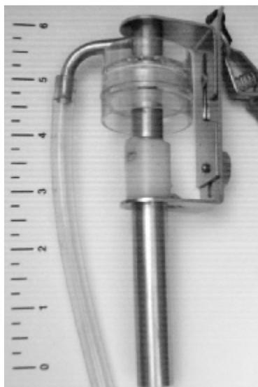
**Figure 2g.** Dorr-Oliver 10-mm nylon cyclone. Used as a respirable sampler most often at 1.7 L/min. A version of this sampler is used at 2 L/min in coal mines with a 1.38 correction factor applied to the resultant mass. The holder encases body of the cyclone so that only the inlet section is visible just below the connection to the 37 mm cassette. The coal mine dust sampler version uses a cassette with an aluminum cartridge encasing the collection filter.
