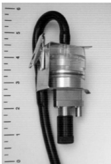
**Figure 2h.** Higgins-Dewell cyclone. Developed and used primarily as a respirable sampler in the UK. This version provides an interface directly to a 37-mm cassette. Cyclone construction is steel and operates at 2.2 L/min.
