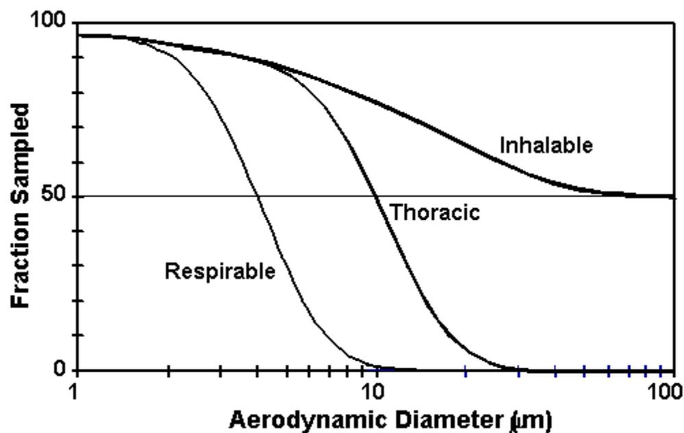
**Figure 1.** ISO/ACGIH/CEN sampling conventions. An ideal sampler should have a sampling efficiency curve that matches one of these curves as closely as possible under all wind directions and velocities. The 50% cutpoints for the respirable and thoracic conventions are 4 and 10  $\mu\text{m}$  respectively.
