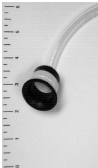
**Figure 2f.** Bell mouth cowl sampler. An alternative to the standard asbestos sampling cassette. The inlet is flared to reduce the effect of external air motion on sample uniformity. Made of conductive plastic and is operated at a flow rate between 0.5 L/min to 16 L/min.
