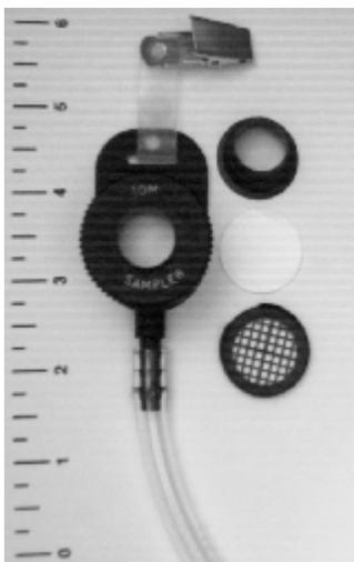
**Figure 2b.** IOM inhalable sampler. This is the first sampler designed specifically to match the inhalable sampling convention. The sampling cartridge is shown on the right with the inlet, filter, and support grid from top to bottom. All dust entering the cartridge is collected and analyzed. Sampler is made of conductive plastic and operates at 2 L/min.
