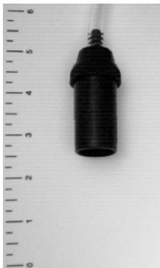
**Figure 2e.** Asbestos sampling cassette. The long (50 mm) inlet was designed to prevent incidental contact with the filter surface and, when facing downward, acts to a certain extent as an elutriator, preventing larger particles from reaching the filter surface. Made of conductive plastic and is operated at a flow rate between 0.5 L/min to 16 L/min.
