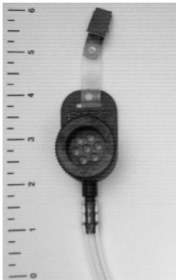
**Figure 2c.** Seven hole sampler used for inhalable dust sampling in the UK. Sampler is made of conductive plastic and operates at 2 L/min.
