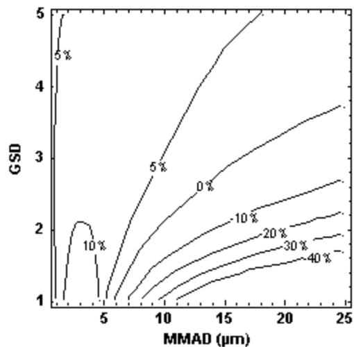
**Figure 3.** Bias map for the 10-mm nylon cyclone (operated at 1.7 L/min) compared with the respirable convention [33]. The contour lines represent percent bias for specific lognormal size distributions. The calculation of this map is based on laboratory measurement of cyclone penetration and can be used with measured field size distributions to estimate sampling bias.
