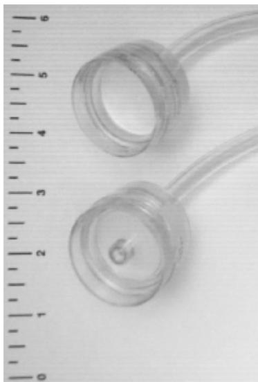
**Figure 2a.** Examples of personal aerosol samplers. a. Open faced (top) and closed face (bottom) 37 mm cassette samplers. These are shown in acrylic copolymer (clear, non-conducting) material and are more prone to electrostatic losses. Other construction materials are available, including conducting plastic. Sampling flow rates range from 0.5 to 10 L/min.
