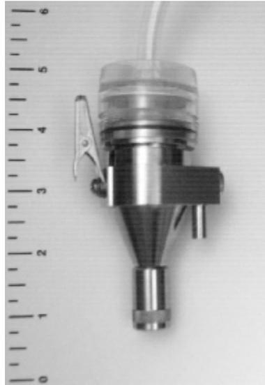
**Figure 2i.** GK2.69 cyclone. This cyclone was designed to match the slope of the thoracic and respirable conventions more closely than other sampling cyclones. Cyclone construction is stainless steel and operates at 4.2 L/min as a respirable sampler and 1.6 L/min as a thoracic sampler.
