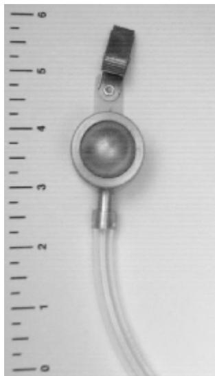
**Figure 2d.** Button sampler. So-named because the inlet, a hemispherical screen with  $\sim 380 \mu\text{m}$  diameter holes, resembles a large button. Developed as an inhalable sampler with reduced wind direction response and improved filter deposit uniformity. Uses metal construction and operates a 4 L/min.
