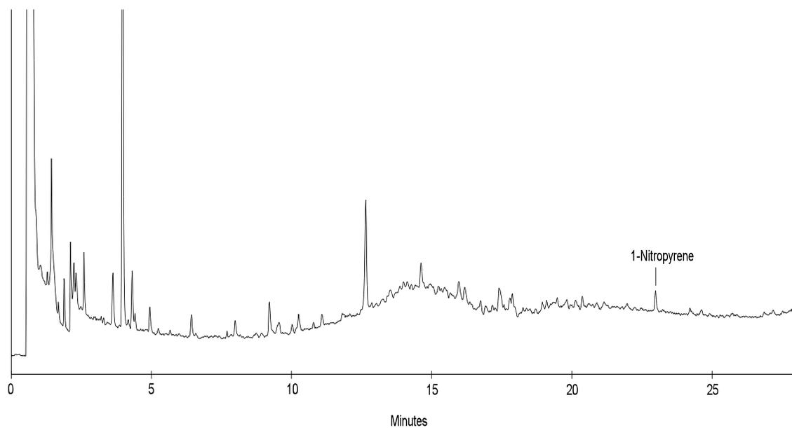
**FIGURE 2:** The chromatogram shown here is from the analysis of the NIST SRM-1650 Diesel Particulates. The diesel particulate, 2.10 mg, was weighed on a glass fiber filter and carried through the complete sample extraction and preparation procedure. The quantity of 1-nitropyrene in this sample was 39.9  $\mu\text{g}$ .
