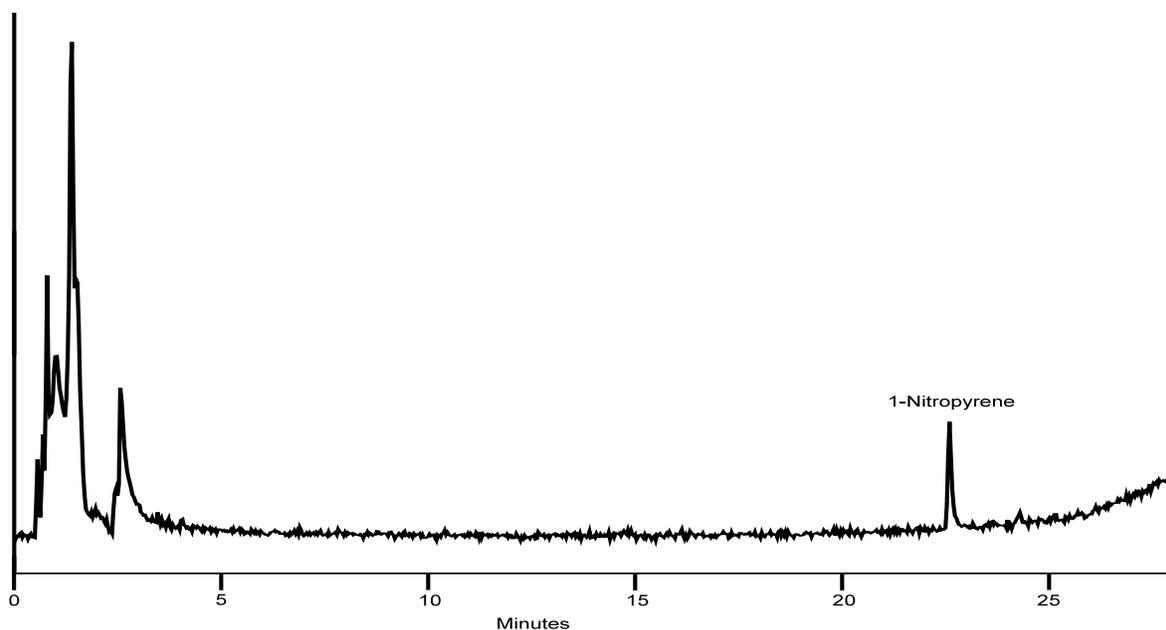
**FIGURE 1:** This is a chromatogram of a 1-nitropyrene 60 ng standard. The major peak at approximately 22.5 minutes is 1-nitropyrene. This chromatogram shows some hydrocarbon response and a baseline with a higher than normal noise level due to the effort to obtain as much sensitivity as possible for samples in the low nanogram region.
