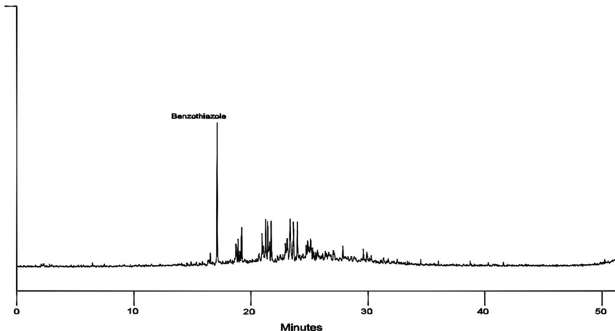
**FIGURE 1:** This is a chromatogram from the analysis of benzothiazole in an asphalt fume sample. The major peak at approximately 18 minutes is benzothiazole. In many cases, the sample matrix may not be this complex and the chromatographic conditions can be adjusted to suit the analysis needs.
