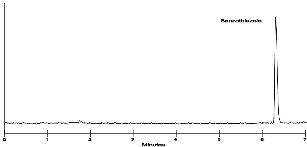
**FIGURE 2:** The chromatogram shown here is a typical chromatogram from the analysis of a desorbed laboratory spiked ORBO-43 sampling tube. The chromatographic conditions have been altered to give a shorter retention time for the benzothiazole because there are no other interfering compounds present.
