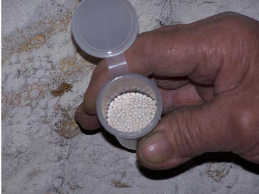
Figure C1. Sample tube containing molecular sieves.
