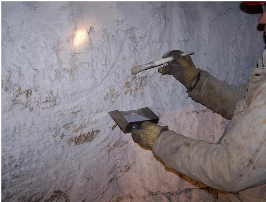
**Figure C2. Collecting a band sample.**
