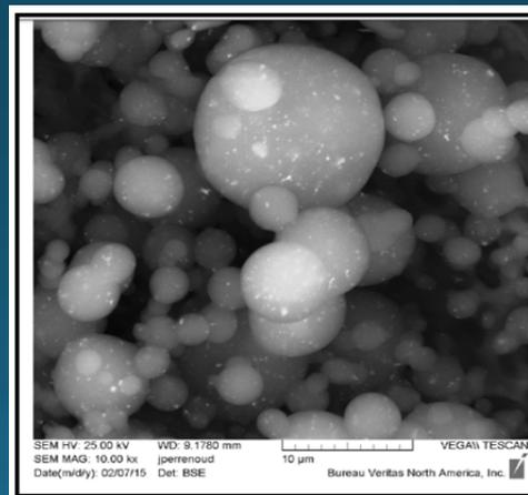
ZnO particles on paint droplets
