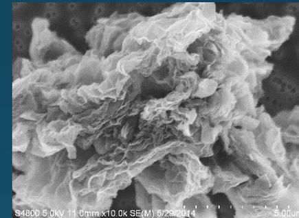
Layered Reduced Graphene Oxide
