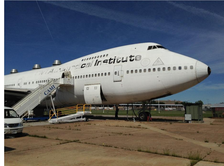
The FAA's Boeing 747 test aircraft used to do a 3-D scan of the cabin and create a lab mock-up cabin
