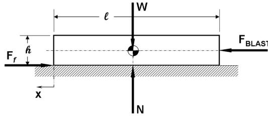
Figure 1: Free Body Diagram of Chamber
