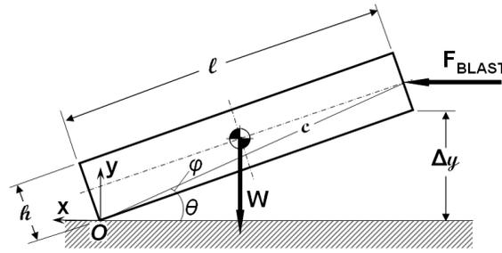
Figure 3: Chamber undergoing rotational displacement
