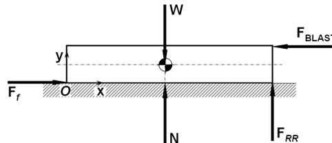
Figure 4: Rotational restraining force on chamber
