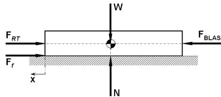
Figure 2: Translational restraining force on chamber
