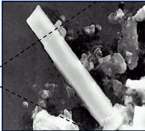
“The fiber shown has a length of nearly 22 microns and a width of almost 3.4 microns, said Dr. Robert Fisher, president and chief scientist at Lab/Cor. This length-to-width ratio of 6.4 to 1 means that according to EPA protocol, this fiber must be counted as asbestos....”
