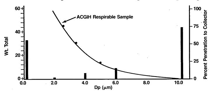
Optical Sizing Results (11 Respirable Dust Samples)
