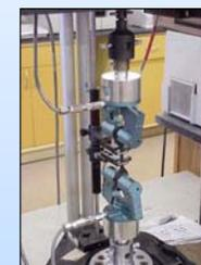
Tensile Strength Test
