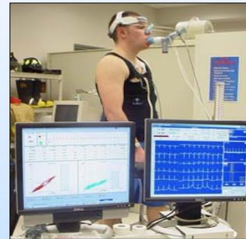
Figure 2. Test subject in the physiology lab wearing the sensor vest and making metabolic measurements
