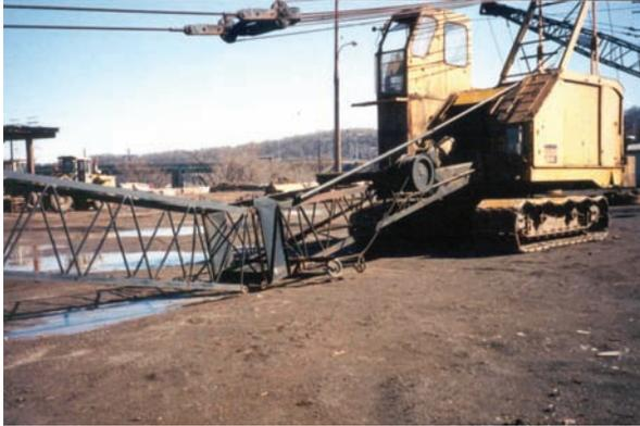
**Figure 7.** Boom collapse during crane disassembly.
